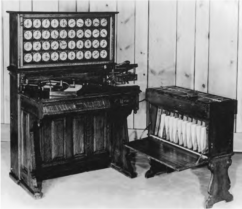
The Hollerith tabulator. Designed for the United States Census, it was a breakthrough in electric data processing equipment. (Courtesy of IBM Corporate Archives)
