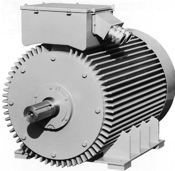
Plate 1.2 Steel frame cage induction motor, 150 kW (201 h.p.), 1485 rev/min. The active parts are totally enclosed, and cooling is provided by means of an internal fan which circulates cooling air round the interior of the motor through the hollow ribs, and an external fan which blows air over the case. (Photograph by courtesy of Brook Crompton.)
