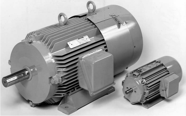
Plate 3.2 Totally-enclosed fan-ventilated wound-field d.c. motors. The smaller motor is rated at 500 W (0.67 h.p.) at 1500 rev/min, while the larger is rated at 10 kW (13.4 h.p.) at 2000 rev/min. Both motors have finned aluminium frames. (Photograph by courtesy of Brook Crompton)
