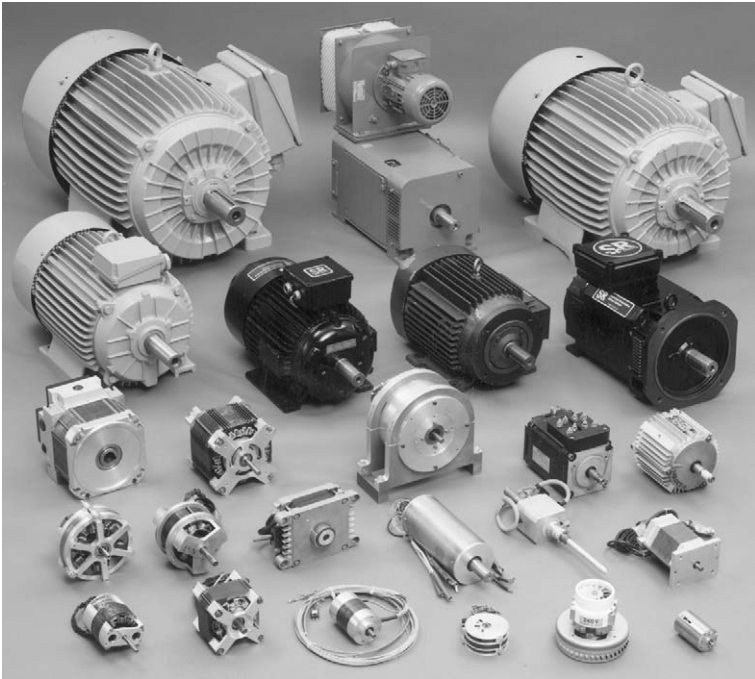
Plate 10.1 Switched reluctance motors. The motors with finned casings are TEFV for use in general-purpose industrial controlled speed drives, the largest being rated at 75 kW (100 h.p.) at 1500 rev/min. The force-ventilated motor (centre rear) is for high-performance ('d.c. equivalent') applications. Most of the other motors are designed for specific OEM applications, including domestic white goods (left front) automotive (centre front), food processor and vacuum cleaner (right front). Very high speeds can be used because the rotor is very robust and there are no brushes, and thus very high specific outputs are obtained; some of the small motors run at up to 30 000 rev/min. (Photograph by courtesy of Switched Reluctance Drives Ltd)
