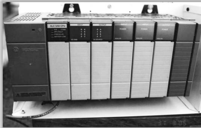
Fig. 12.4 Photographic view of Allen Bradleys Modular type PLC and Input/Output modules.
