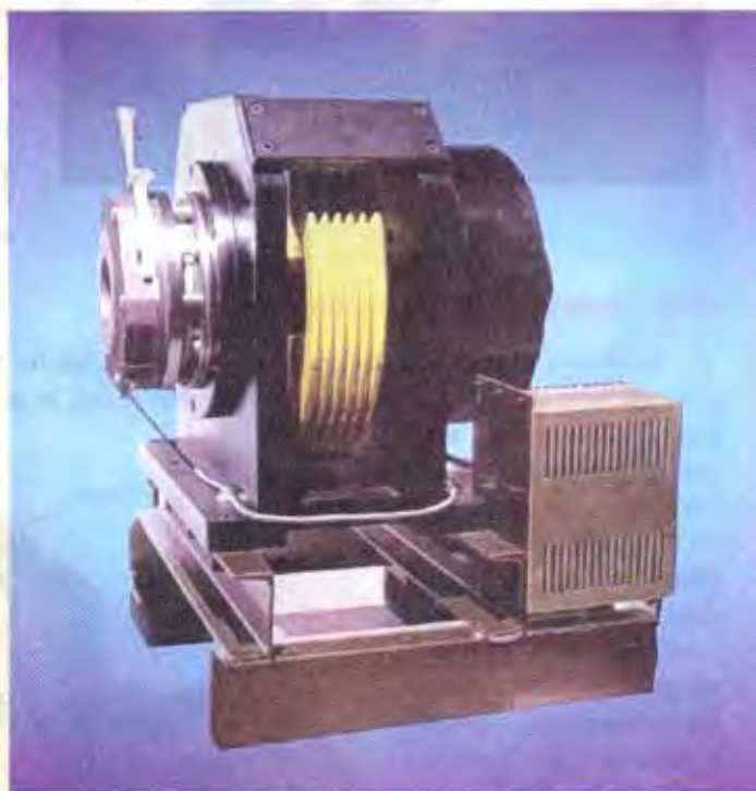
Rotary synchronous motor for lift applications
