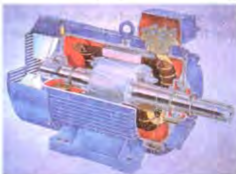
Fig. 34.1 Squirrel cage AC induction motor opened to show the stator and rotor construction, the shaft with bearings, and the cooling fan.
