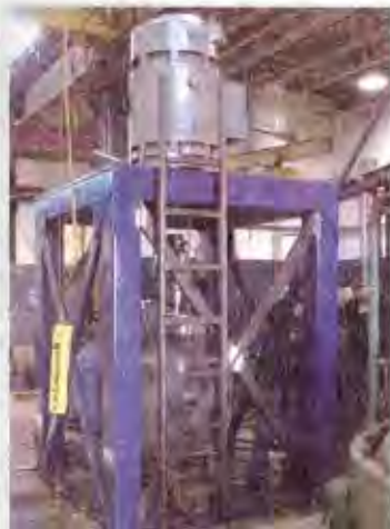
This vertical test stand is capable of absorbing up to 10,000 N-m of torque at continuous load rating (max 150.0 hp at 1800 rpm). It helps to develop speed torque curves and performs locked rotor testing
