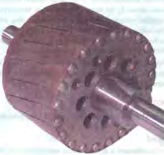
Salient - poled squirrel cage motor
