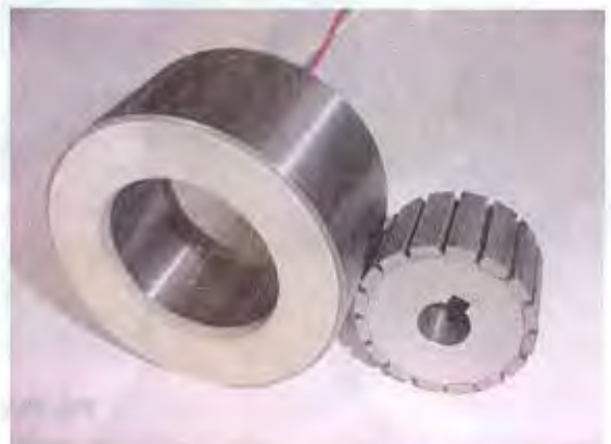
Permanent magnet stepper motor
