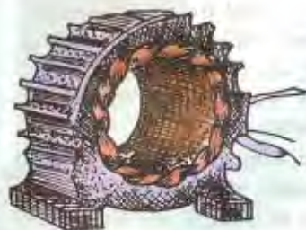
Fig. 34.2 (b) Completely wound stator for an induction motor. (Courtesy : Gautam Electric Motors)
