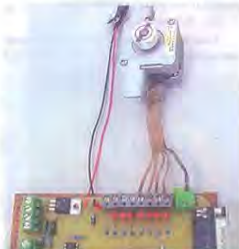
Connecting a stepper motor to the interface
