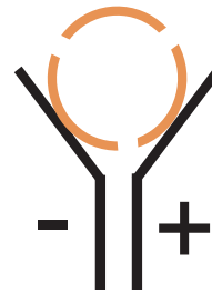
commutator orientation when coils are conducting
