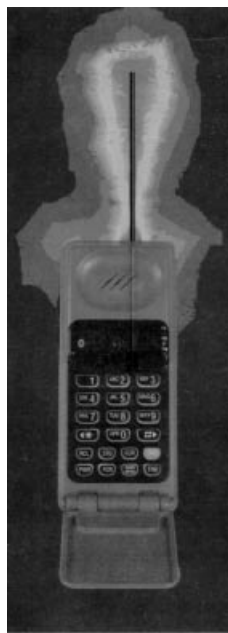
Figure 1-1 Simulated antenna radiation of a Motorola flip phone.
