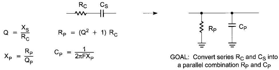
Figure 3-114 Converting from series to parallel configuration.
