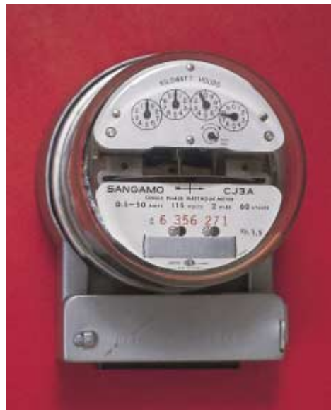
FIGURE 4–21 Watt-hour meter. This type of meter uses a gear train to drive the dials. Newer meters are electronic with digital readouts.
