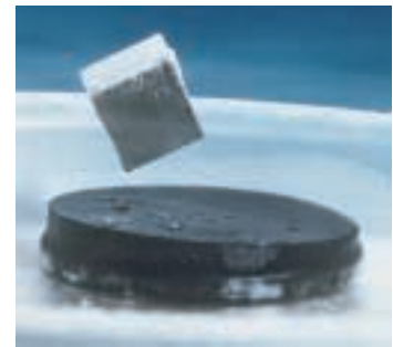
FIGURE 3–31 The Meissner effect: A magnetic cube hovers above a disk of ceramic superconductor. The disk is kept below its critical temperature in a bath of liquid nitrogen. (Courtesy of AT&T Bell Laboratories/AT&T Archives)
