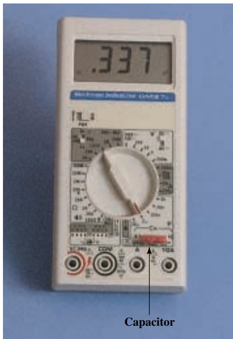
(a) Measuring C with a DMM. (Not all DMMs can measure capacitance)
