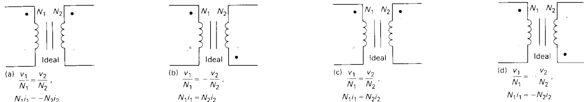
FIGURE 13.19 Circuits that show the proper algebraic signs for relating the terminal voltages and terminal currents of the ideal transformer.
