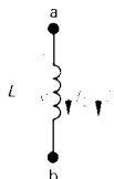
FIGURE 16.2 An inductor of L henrys carrying an initial current of i_0 amperes.
