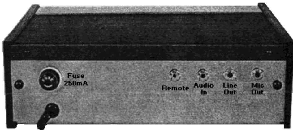
ScanMate viewed from the back. The fuse as well as the Remote, input, Mic-output, Line-out and Audio input jacks are located on the rear panel of the enclosure. All connections to and from the ScanMate's unit are through those jacks.
