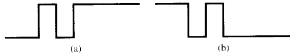
Figure 3.31 Dynamic hazards. (a) Dynamic hazard on 0 to 1 change. (b) Dynamic hazard on 1 to 0 change.
