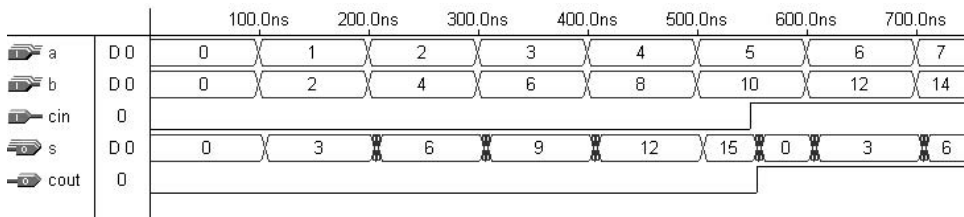
Figure 9.7 Simulation results from the carry ripple adder of figure 9.6.
