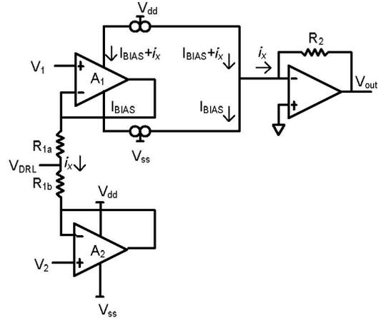
Fig. 3. Schematic of INA.
