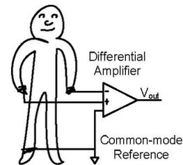
Fig. 1. Typical measurement of biopotentials.
