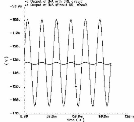
Fig. 9. Effect of output voltage with DRL and without DRL.
