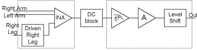
Fig. 2. Block diagram of the ECG measurement circuit
