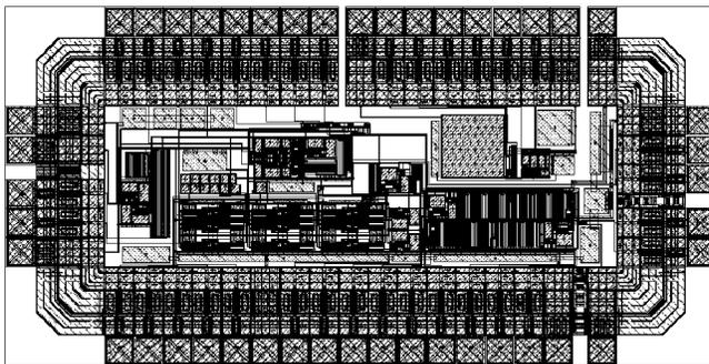
Fig. 13. Layout of the ECG IC.
