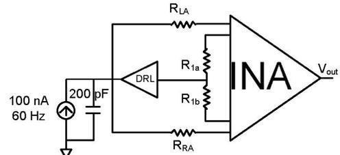
Fig. 8. Simulation setup for testing the DRL.
