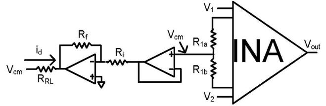
Fig. 4. Driven-Right-Leg circuit
