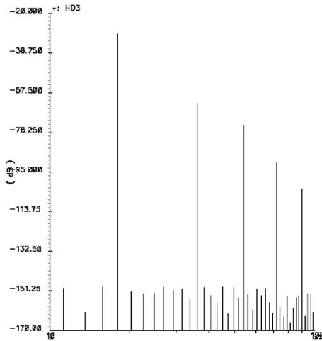
Fig. 11. Simulated harmonic distortion components for the filter.
