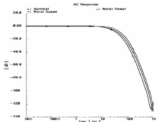
Fig. 10. Frequency response of Gm-C LPF in the presence of temperature and process variation
