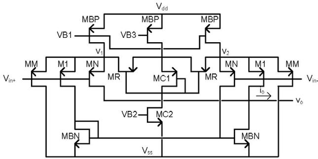
Fig. 5. Schematic of OTA
