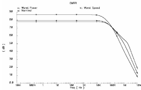
Fig. 7. Worst case and nominal simulation of CMRR of INA.
