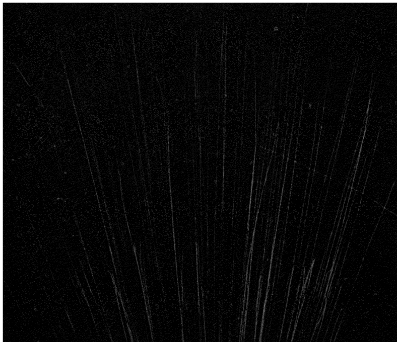
Fig 5 — Cloud-track photograph showing the transmutation of a nitrogen nucleus by the capture of an \alpha -particle and emission of a proton (after Blackett)
