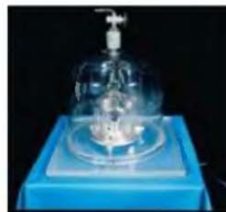
1.4 The metal object carefully enclosed within these nested glass containers is the international standard kilogram.
