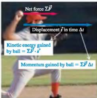
8.4 The kinetic energy of a pitched baseball is equal to the work the pitcher does on it (force multiplied by the distance the ball moves during the throw). The momentum of the ball is equal to the impulse the pitcher imparts to it (force multiplied by the time it took to bring the ball up to speed).
