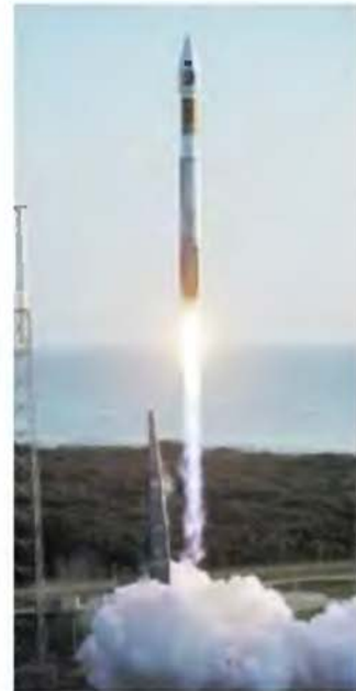
8.33 To provide enough thrust to lift its payload into space, this Atlas V launch vehicle exhausts more than 1000 kg of burned fuel per second at speeds of nearly 4000 m/s.
