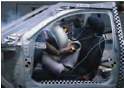
8.2 If a fast-moving automobile stops suddenly in a collision, the driver's momentum (mass times velocity) changes from a large value to zero in a short time. An air bag causes the driver to lose momentum more gradually than would an abrupt collision with the steering wheel, reducing the force exerted on the driver as well as the possibility of injury.
