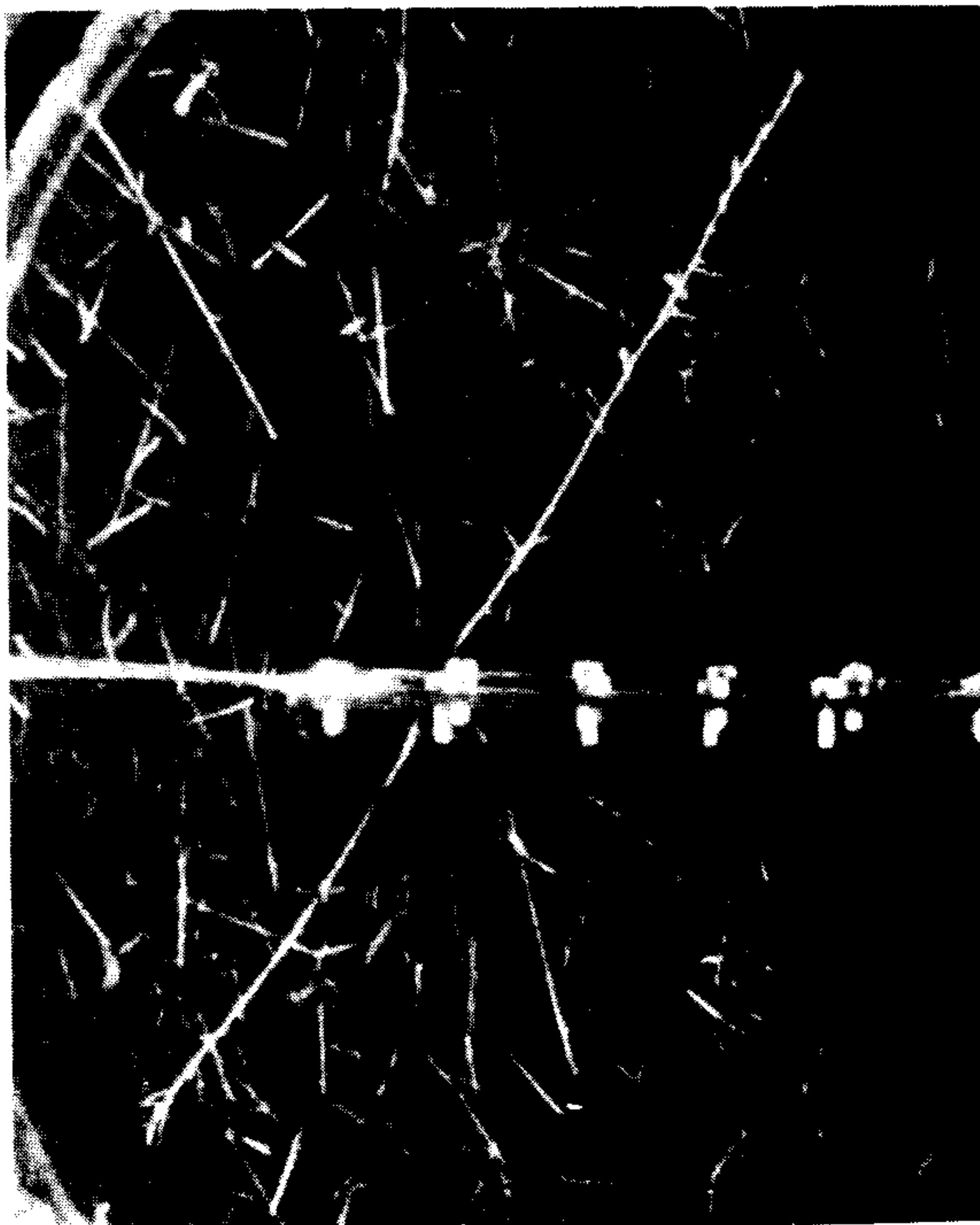
Fig. 9-14. Cloud-chamber photograph of the tracks of the two fragments resulting from the fission of a uranium nucleus [Bøggild, Brostrøm, and Lauritsen, Phys. Rev. 59 , 275 (1941)]. Initially the uranium nucleus was at rest in the thin horizontal metal plate at the center of the photograph. The two fragments move in opposite directions. From the analysis of the paths, we can estimate the energies of the fragments, which in turn (using the relation derived in Example 9.12) allow us to obtain the ratio of their masses. The effect of the neutrons released is neglected.
