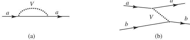
Fig. 5.10. Diagram showing the world-lines of: (a) particle a emitting and reabsorbing a V boson; (b) particles a and b exchanging a V boson.
