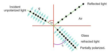
**Fig. 15.36** Polarization by reflection  $\bullet$   $\sigma$ -component  $\leftrightarrow \pi$ -component
