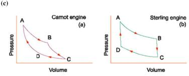
**Fig. 10.12** (a) Carnot cycle consisting of two isothermic processes AB and CD; two adiabatic processes BC and DA. (b) Sterling cycle consisting of two isothermic process AB and CD, two isochoric processes BC and DA
