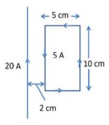
**13.58** (a) A very long straight wire PQ of negligible diameter carries a steady current  $I_1$ . A rigid square coil ABCD of side l and n turns is set up with sides AB and DC parallel to the coplanar with PQ as shown in Fig. 13.16. The side of the coil AB is at distance d from the wire PQ. Derive an expression for the resultant force on the coil when a steady current  $I_2$  flows through it. What is the direction of the force?
