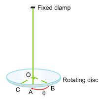
its original position. For small twists the restoring torque will be proportional to the angular displacement in accordance with Hooke's law.
