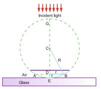
**Fig. 15.32** Newton's rings with convex lens on a flat surface
