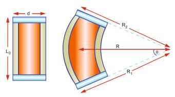
Fig. 10.2 Expansion of a bimetal strip of bars
