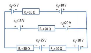
**12.55** Apply Kirchhoff's rules to the circuit shown in Fig. 12.29 and present the simultaneous equations necessary to calculate the currents in each of the branches of the circuit. You do not have to solve these equations for the branch currents.
