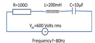
(iv) Find the phase angle between supply voltage and current through the circuit.
