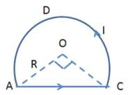
**13.27** (a) A current *I* is sent through a thin wire as in Fig. 13.6. The straight wires are very long and the radius of the curved part of the wire is *R*. Show that the magnetic induction at the point O will be
