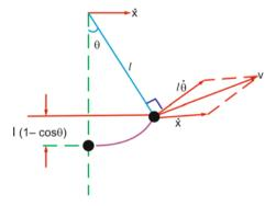
The velocity v of the bob is obtained by combining vectorially its linear velocity  $(l\dot{\theta})$  with the velocity of the block  $(\dot{x})$ . The height through which the bob is raised from the equilibrium position is  $l(1-\cos\theta)$ , where l is the length of the pendulum:
