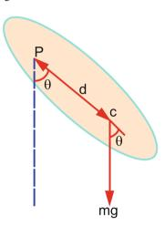
The body is pivoted to a horizontal frictionless axis through P and displaced from the equilibrium position by an angle  $\theta$ . In the equilibrium position the centre of mass C lies vertically below the pivot P. If the distance from the pivot to the centre of mass be d, the mass of the body M and the moment of inertia of the body about an axis through the pivot I, the time period of oscillations is given by
