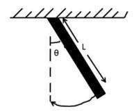
uniform rod about one end is  $I = \frac{1}{3}ML^2$ , obtain an equation for the period of the oscillatory motion for small angles. What would be the length l of a simple pendulum that has the same period as the swinging rod?
