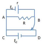
12.32 A thin uniform wire 50 cm long and of  $1\,\Omega$  resistance is connected to the terminals of an accumulator of emf 2.2 V and the internal resistance 0.1  $\Omega$  (Fig. 12.17). If the terminals of another cell can be connected to two points 26 cm apart on the wire without altering the current in the wire, what is the emf of the cell?
