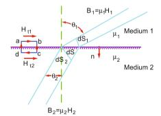
**Fig. 14.8** The refraction of magnetic lines
