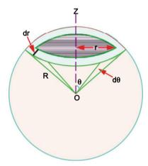
Consider a circular strip of radius r and width dr, symmetrical over the sphere's surface. The angle  $\theta$  is measured with respect to the z-axis.
