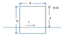
(iii) Obtain an expression for the emf induced in the coil if the wire is placed at x = b/4 and the current varies with time according to I = 2t.
