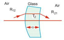
Fig. 15.26 Sequences of refraction, translation and refraction for a thick lens placed in air
