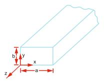
Fig. 14.13 Rectangular hollow metal waveguide
