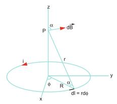
**Fig. 13.26** Magnetic induction on the axis of a current-carrying ring
