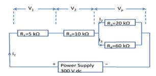
**12.54** Apply Kirchhoff's rules to the circuit shown in Fig. 12.28 to produce three equations with three unknown branch currents. You do not have to solve these equations for individual I.
