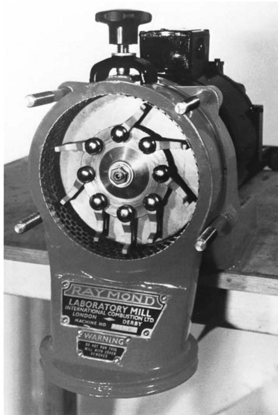
Figure 2.10. The Raymond laboratory hammer mill
