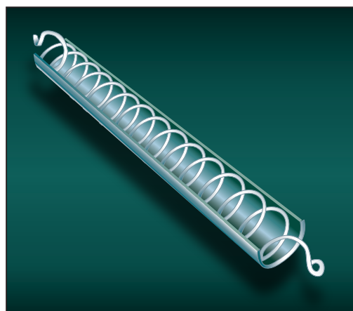
FIGURE 4. The use of a full-length, helically coiled insert can increase the swirl and pressure gradient in the radial direction
