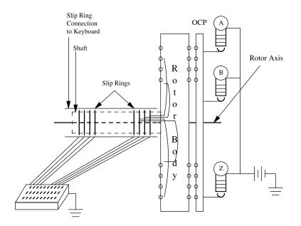
Figure 7.1 A half-rotor cryptomachine schematic.
