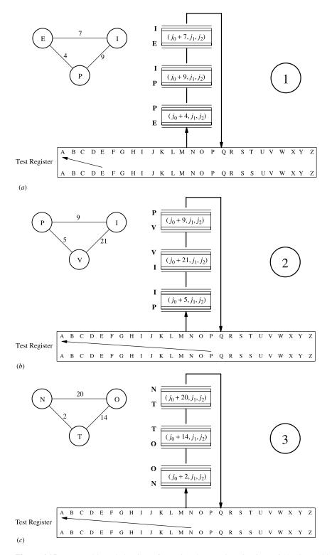
**Figure 6.15** (*a*) Double-ended Enigma for testing the EPI-loop in Figure 6.12; (*b*) Double-ended Enigma for testing the VIP-loop in Figure 6.12; (c) Double-ended Enigma for testing the NOT-loop in Figure 6.12.
