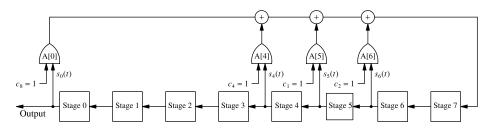
Figure 8.8 The LFSR determined in *Example 8.7* cribbing.
