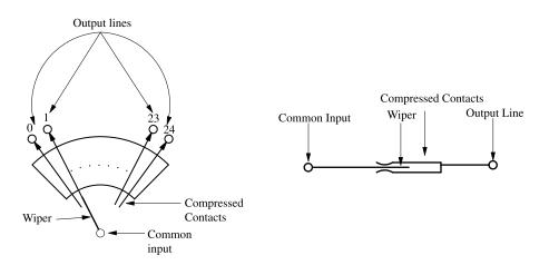
Figure 7.5 Side and top view of stepping switch.
