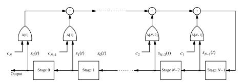
Figure 8.2 Linear feedback shift register.
