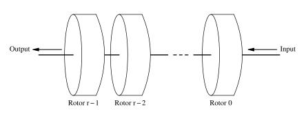
Figure 6.3 A straight-through rotor system.
