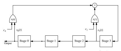
**Figure 8.5** The LFSR with characteristic polynomial  $p(z) = 1 + z^3 + z^4$ .
