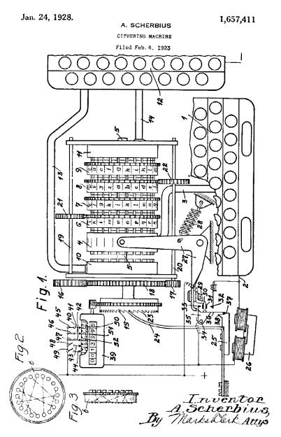
Figure 6.7 U.S. Patent 1,657,411: The Enigma machine.
