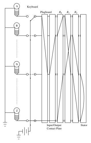
Figure 6.10 The Enigma signal path.
