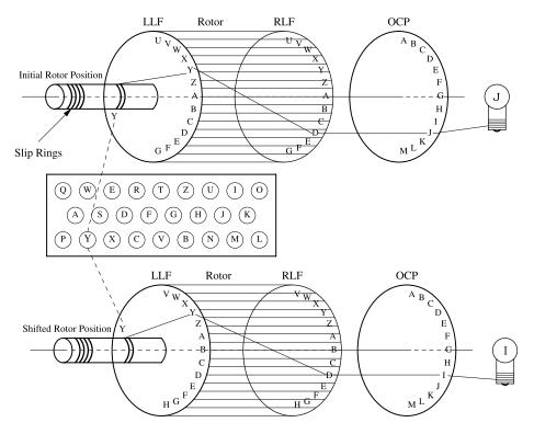
Figure 7.2 Encipherment path with keyboard Y depressed.
