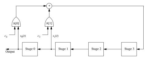
**Figure 8.6** The LFSR with characteristic polynomial  $p^*(z) = 1 + z + z^4$ .
