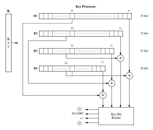
Figure 9.19 Key control block Cipher system.
