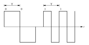
Figure 18.2 F2F (Two frequency recording).
