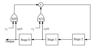
**Figure 8.4** The LFSR with characteristic polynomial  $p(z) = 1 + z + z^3$ .
