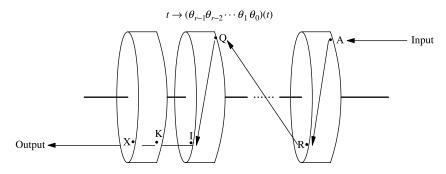
Figure 6.4 An encipherment path in a straight-through rotor system.
