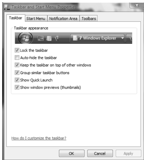
FIGURE 4.2 The Taskbar tab of the Taskbar and Start Menu Properties dialog box
