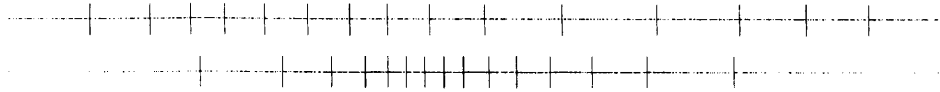
Figure 19.7: Quantization thresholds found by the scalar quantization algorithm for uniform and Gaussian distributed data. For both cases 1000 points were generated, and 16 centers found by running the basic scalar quantization algorithm until convergence.
