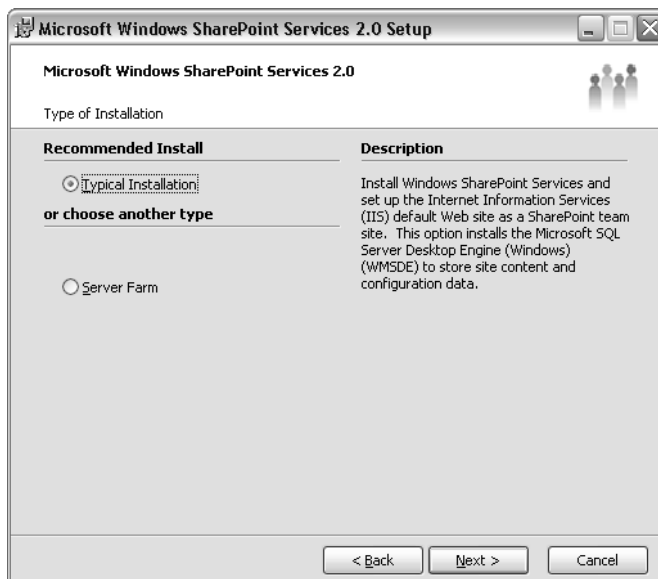
Figure 13-10. A server farm installation installs Windows SharePoint Services and a Central Administration server. A typical installation also installs WMSDE, creates configuration and content databases, and extends the default Web server.
