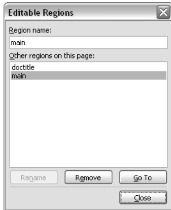
Figure 9-11. This dialog box marks the current Design view selection as an editable region and gives the region a name.
