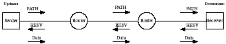
Figure 9-6 PATH and RESERVATION (RESV) messages in RSVP
