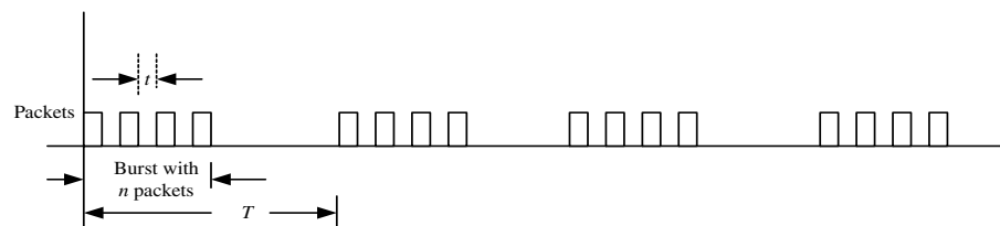
Figure 9-9 An overly simplified traffic pattern used in calculating bandwidth in admission control
