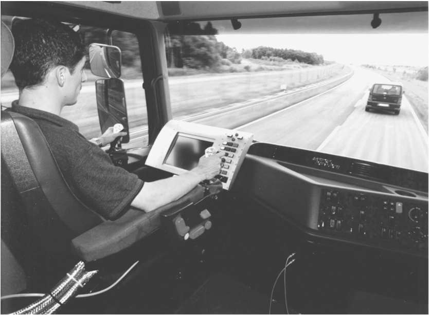
FIGURE 16.11 Side stick control of a truck (Daimler-Chrysler).
