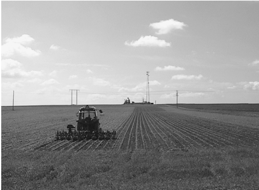
Figure 7. Field test of the row-recognition system with a tractor and a row-cultivator removing weed between the rows.
