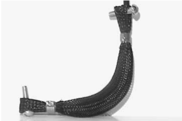
■ 16.5 Screw going through one end loop of air muscle
