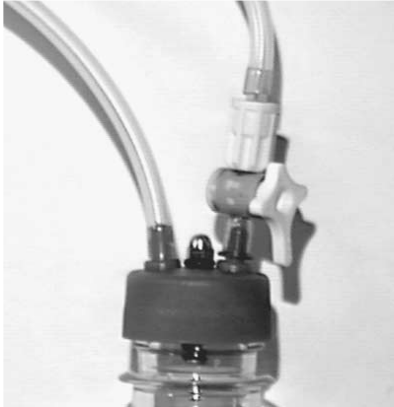
■ 16.11 Using clear plastic tubing on standard adapters
