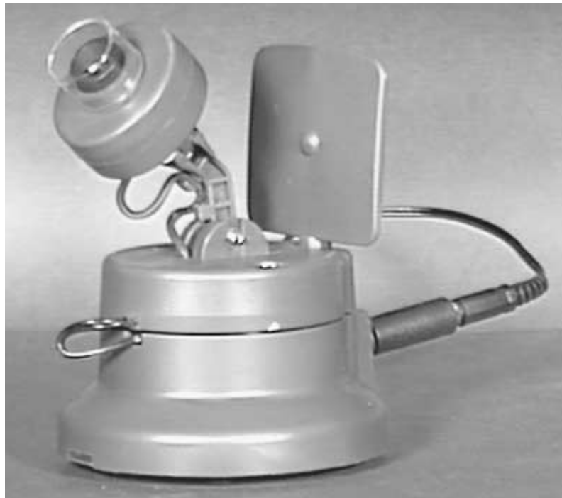
■ 9.7 Color camera with battery pack ready for mounting on R/C car
