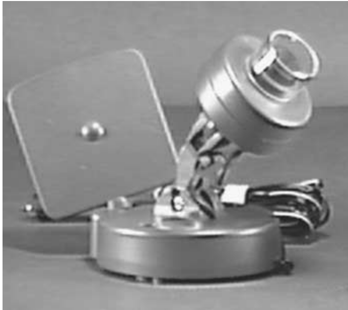
■ 9.4 Color camera with audio and 2.4-GHz transmitter
