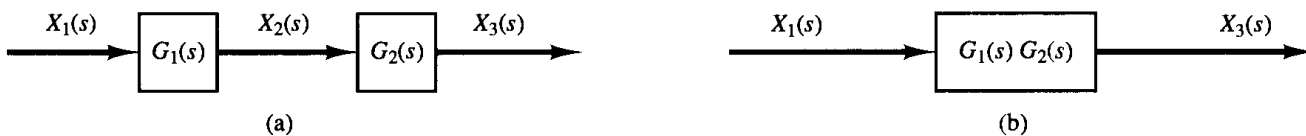
Figure 3–20 (a) System consisting of two nonloading cascaded elements; (b) an equivalent system.
