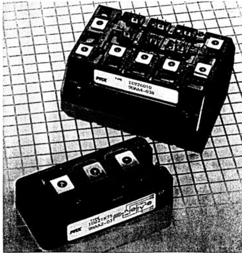
FIGURE 3-19 Transistor modules that show the terminal layout. The terminals in this module match the diagram shown in Figs. 3-16 and 3-18. (Courtesy of POWEREX Inc.)
