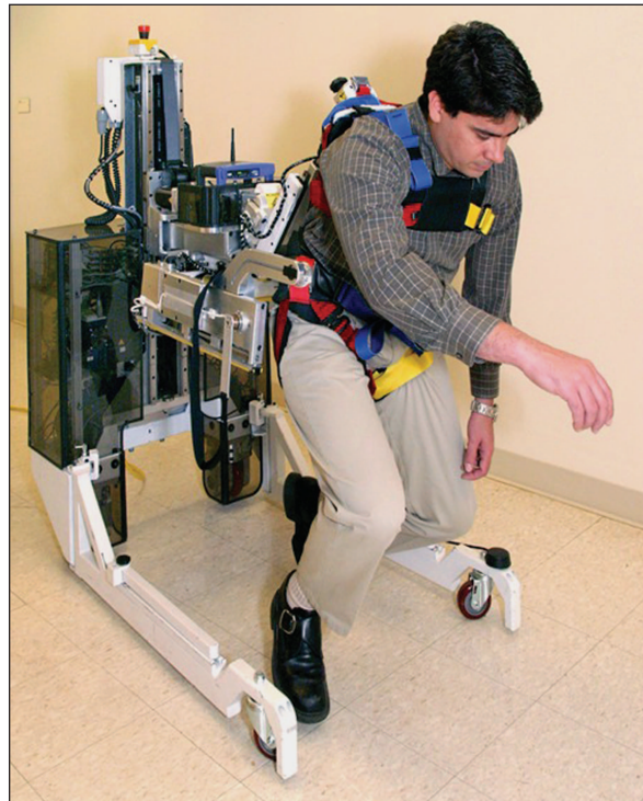
The KineAssist robotic device helps retrain muscles and nerves after a stroke or accident. (Photo courtesy of the Rehabilitation Institute of Chicago.)
