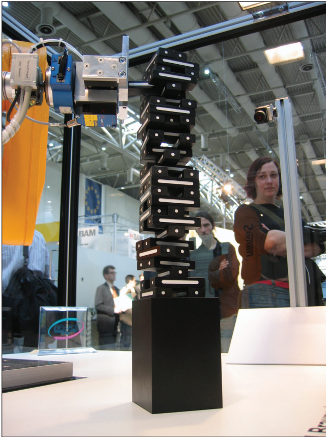
Figure 4. Jenga-playing manipulator with a tower of 27 levels. Videos of this project can be found in [31] and [35].
