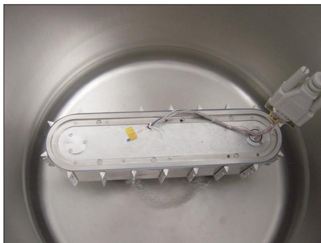
**Figure 4.** Cryogenic test setup of a new track seal prototype.
