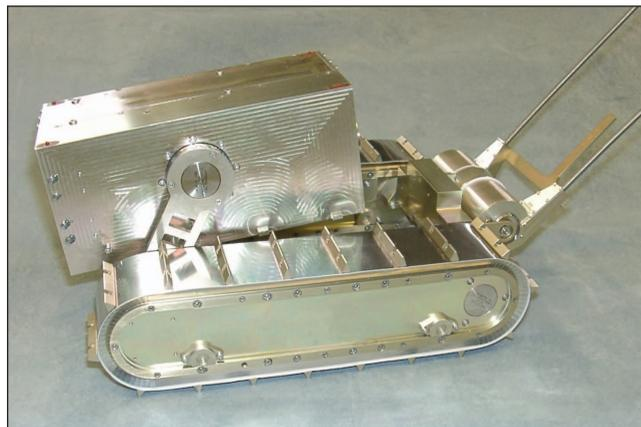
Figure 1. The Nanokhod engineering qualification model (courtesy ESA).
