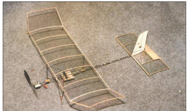
Figure 3. Our 30-g prototype with a 60-cm wingspan flies at speeds of 2 m/s.
