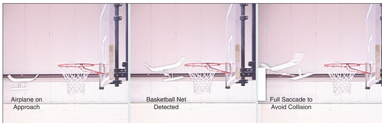
Figure 7. Optic flow is used to sense when an obstacle is within two turning radii of the aircraft. The aircraft avoids the collision by fully deflecting the rudder.
