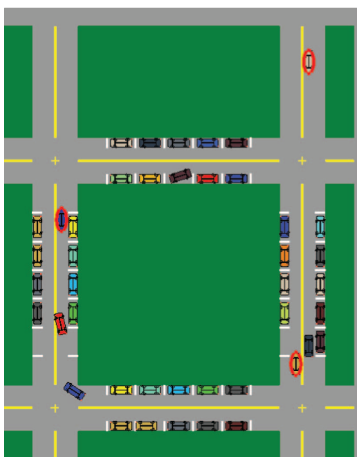
Figure 5. A snapshot of the simulation. Cars surrounded by red ellipses are cars that are stopping because of the hazard input, in this case based on a stoplight.
