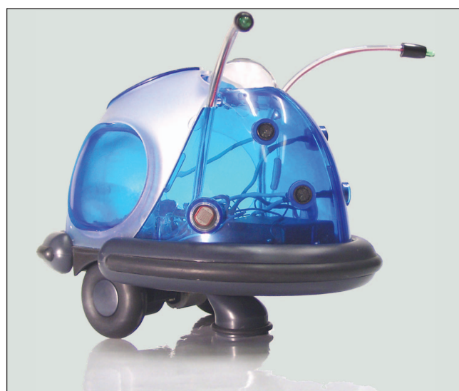
Figure 3. Fully constructed Cybot (25 × 18 × 17 cm) from the parts provided with Issues 1–17 of Ultimate Real Robots Magazine. Autonomous capabilities include line following, basic flocking, and obstacle avoidance.
