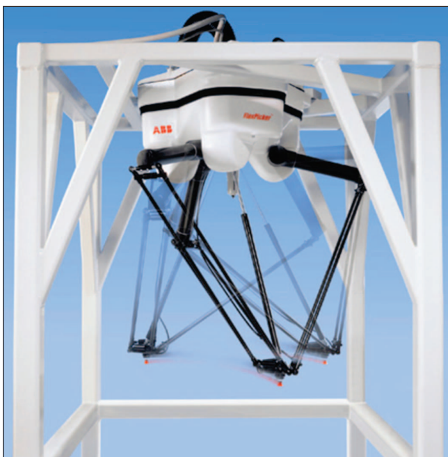
Figure 2. ABB Flexpicker pick-and-place robot, the fastest robot produced by ABB (courtesy ABB).
