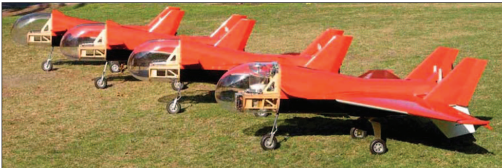
Figure 13. Australian unmanned aerial vehicle fleet with 45-kg aircrafts of 3-m wing spans with reconfigurable sensor payloads (University of Sydney).
