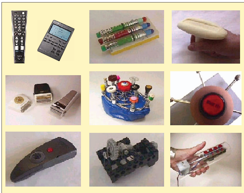
Figure 3. Early prototype for the hand-held media controller project. Found objects and state-of-art examples, Lego + rubber band transmissions, whimsical and serious nonfunctioning concepts, and narrowly targeted functional engineered prototypes.
