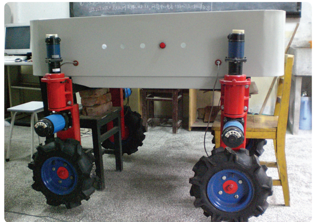
FIGURE 1 An eight-degree-of-freedom autonomous agricultural navigation platform. Each wheel is equipped with a driving motor and a steering motor. Thus, each wheel can be individually steered and driven.
