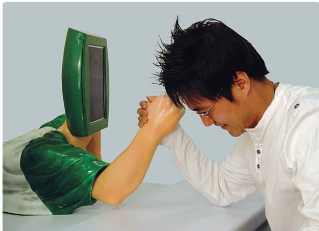
FIGURE 1 The arm-wrestling robot Robo Armwrestler. This robot, which is intended for use in elderly health care, was developed in the Intelligent Control and Robotics Laboratory at Konkuk University in Korea.
