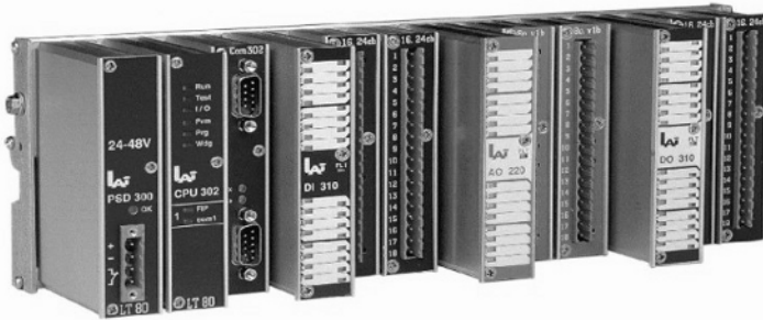
Figure 8.9. PLC Leroy LT160 embedding several RST controllers and I/O modules (courtesy of Leroy Automatismes)
