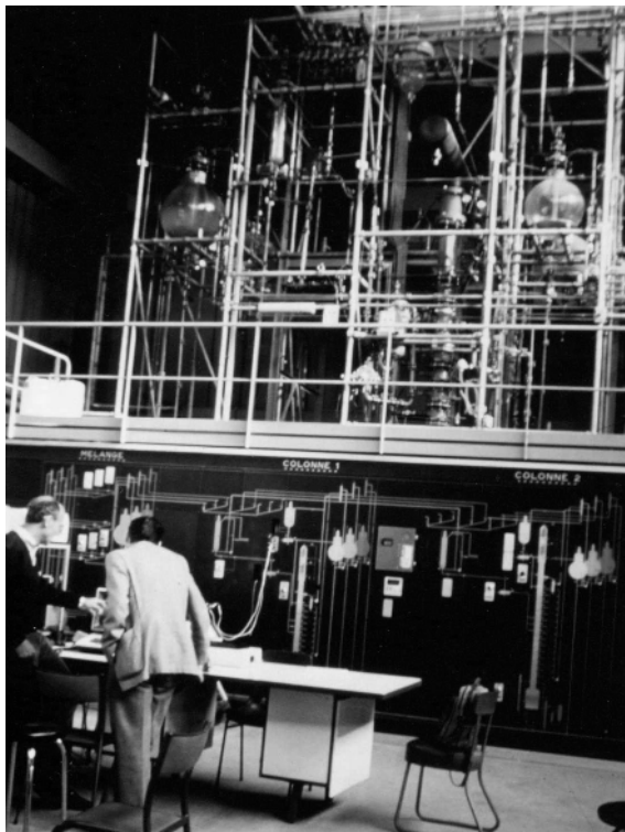
Figure 7.12a,b. Binary distillation column (Laboratoire d'Automatique de Grenoble, INPG/CNRS). a Functional diagram, b View
