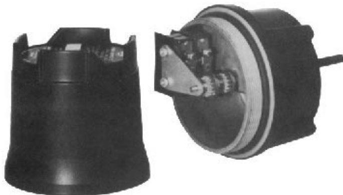
FIGURE 47 Limit switches are common actuator accessories. The unit shown has two limit switches, but similar designs can hold up to six switches and trip points can be adjusted to any point of travel. ( Fisher Controls International, Inc. )
