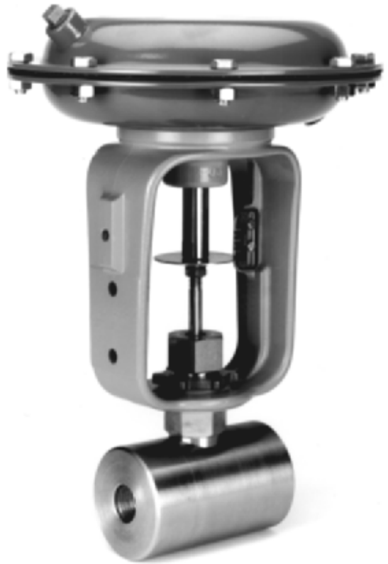
FIGURE 6 Bar-stock valves provide economical solutions to small flow requirements. Pressures to 1500 psig (104 bars) and temperatures to 450°F (232°C) can be handled. Compact spring-and-diaphragm actuators complement these small valve bodies. ( H. D. Baumann Inc. )
