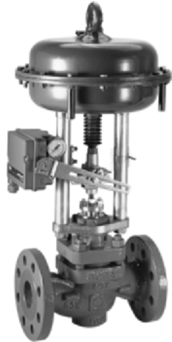
FIGURE 8 Valve style typical of general-purpose valves. Availability usually extends to size NPS 4 or DN 100 and to Class 300 or PN 50 ratings. These valves feature compact, reversible diaphragm actuators and inexpensive positioners. ( Fisher Controls International, Inc. )
