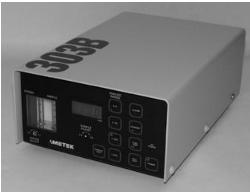
FIGURE 24 Electrolytic P_2O_5 moisture analyzer (courtesy of Ametek).
