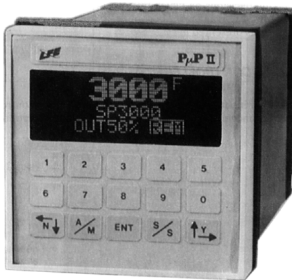
FIGURE 4 Microprocessor-based 1/4 DIN [96 by 96 mm (3.8 by 3.8 in.)] configurable controller. Instrument features blue vacuum fluorescent dot-matrix display (four lines of 10 characters per line), and self-tuning based on one-shot calculation of the optimum PID values based on a “cold” start. Calculated PID values are stored and can be displayed or changed on demand. Both direct- and reverse-acting outputs can be self-tuned. Four PID settings can be stored for each control output. PID set selection may be programmed as part of a profile, initiated by process variable value, internal trigger, keystroke, or logic input signal. Controller uses a dynamic memory rather than fixed allocation of memory. User can assign memory as needed during configuration for best memory utilization. Security by user ID number can be selected at any program level to prevent unauthorized access and program or data changes. Self-diagnostics are used on start-up and during normal operation by monitoring internal operations and power levels. Upon detection of an out-of-tolerance condition, controller shuts off output(s), activates alarm(s), and displays appropriate message. Controller can perform custom calculations using math programs. Device maintains a history file of event triggers as a diagnostic tool. Two process inputs and four outputs can be assigned to two separate control loops creating a dual-loop controller. Optional features include parallel printer output, logic I/O, digital communications, and PC interface. ( LFE Instruments. )
