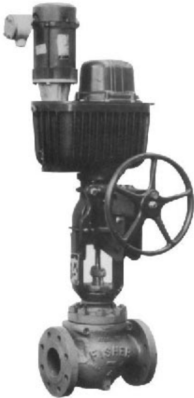
FIGURE 38 Self-contained electrohydraulic actuator. This single unit contains the electric motor, hydraulic pump, reservoir, hydraulic positioner, and actuator cylinder. (Fisher Controls International, Inc.)
