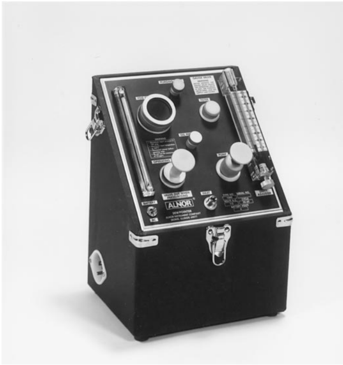
FIGURE 10 Adiabatic expansion or Fog chamber instrument ( courtesy of Alnov ).
