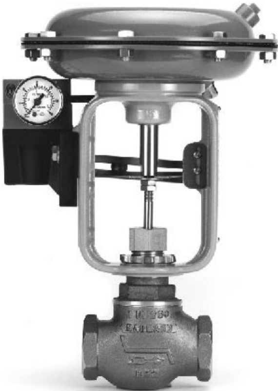
FIGURE 7 Screwed-end bronze valve body capable of handling many utility applications. It is complemented by a wide variety of seat ring sizes and control characteristics. ( H.D. Baumann Inc. )
