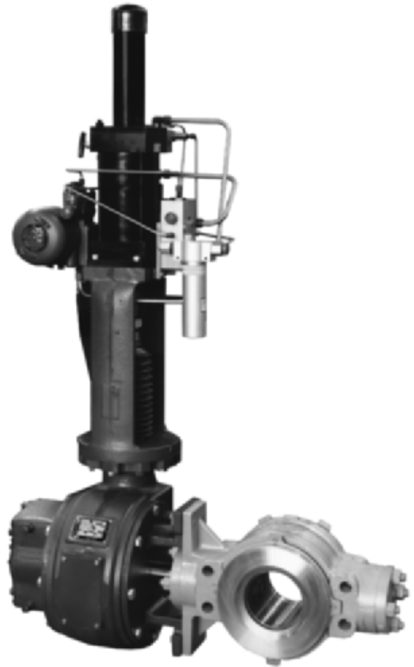
FIGURE 39 Electrohydraulic actuators provide the ultimate in thrust, speed, frequency of response, and stiffness. The type shown is operated by an external hydraulic power supply. (Fisher Controls International, Inc.)
