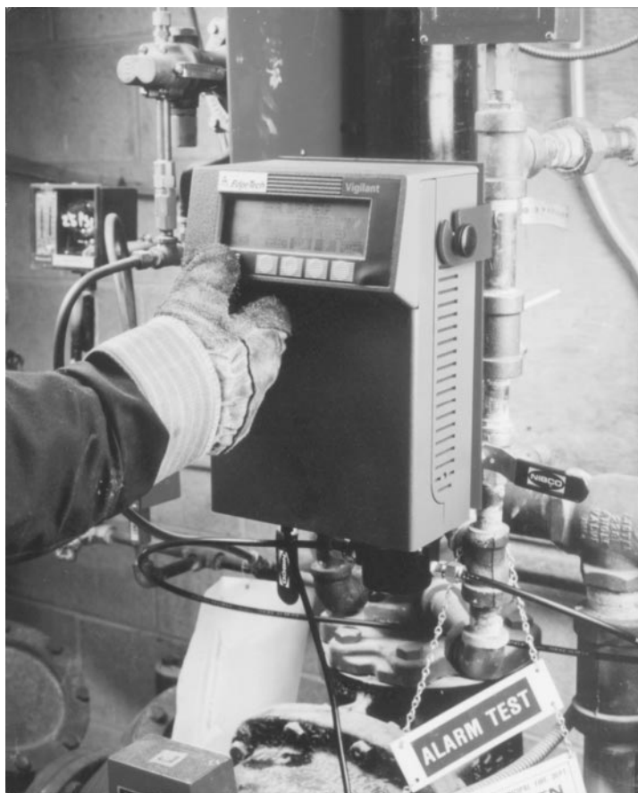
FIGURE 8 Continuous temperature control optical dew point instrument.
