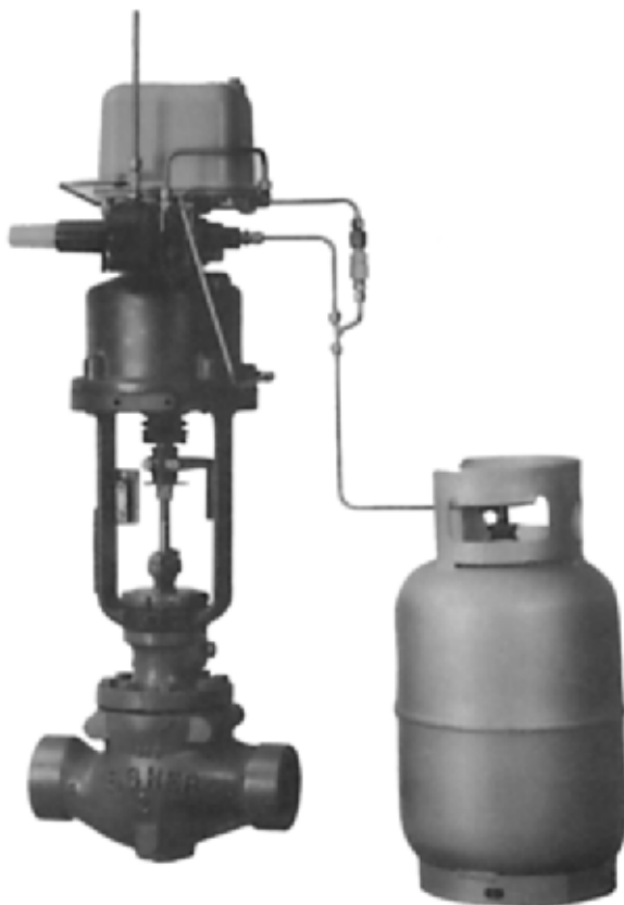
FIGURE 45 Fail action for piston actuators can be accomplished by using pneumatic trip systems. A switching valve transfers stored pressure from volume tanks to the piston to stroke the valve and maintain the predetermined failure position. ( Fisher Controls International, Inc. )
