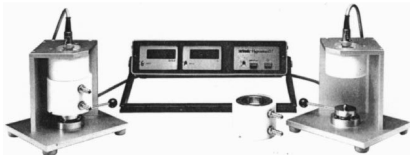
FIGURE 29 %RH instrument for measuring water activity (courtesy Rotronics, Inc.). A relative humidity instrument to measure %RH in the vapor immediately surrounding the specimen to be analyzed. Special containers are included in the system.
