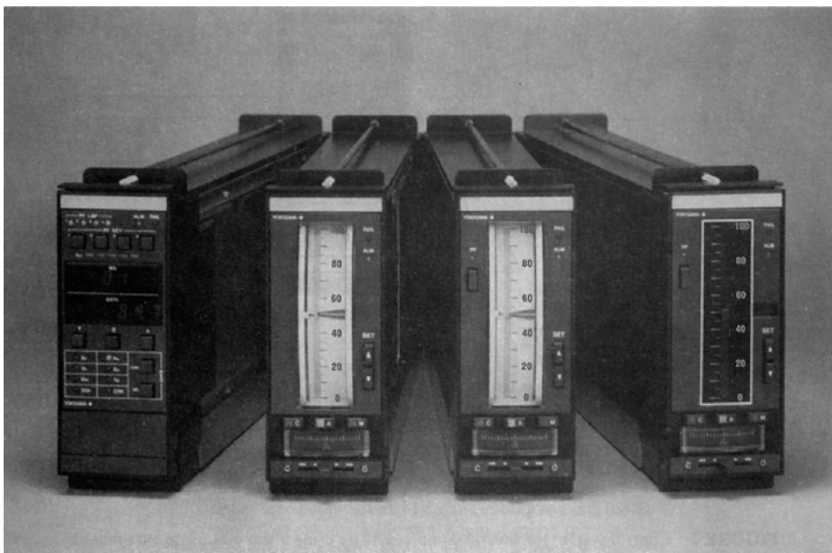
FIGURE 5 Family of single-loop process controllers. These programmable controllers incorporate computational and control functions that can be combined in the same manner as programming a pocket calculator. The self-tuning function for optimizing control is particularly useful in multiproduct batch applications, where process characteristics can vary from product to product. It features a “one-shot” algorithm, triggered by set-point changes or on demand, and provides rapid response to process changes. Other features include feedforward control (with gain and bias computations), signal processing, analog inputs (4 points, 1–5 V dc), analog outputs (3 points, 1–5 V dc; 1 point, 4–20 mA dc). A companion programmable computing station provides data display, signal processing, and sequencing functions. The instrument features 10 status I/O points, each user-definable as input or output. Four programmable function keys on front of panel are used to start control sequences. Four associated lamps indicate sequence progress or serve as prompts. Control period is 0.1, 0.2, or 0.4 s; 500 program steps execute in 0.4 s. There are over 43 computational functions. A device of this kind can control several compressors, for example, as shown in Fig. 6. (Johnson Yokogawa Corporation.)
