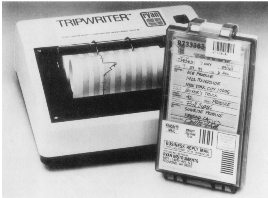
FIGURE 19 Thermistor-based temperature recorder (right) used for monitoring environmental conditions during the transport of various perishable foodstuffs, such as fruits and vegetables, for up to 16 days or more of travel time. These battery-operated units are packaged for mailing. Upon receipt of mailable units, such as Tripmentor TM and Tripwriter TM , user may print out the information on the recorder (left). (Ryan Instruments.)
