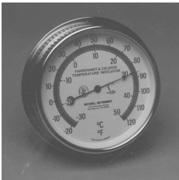
FIGURE 20 Mechanical expansion humidity/temperature indicator (courtesy of Mitchell Instruments).
