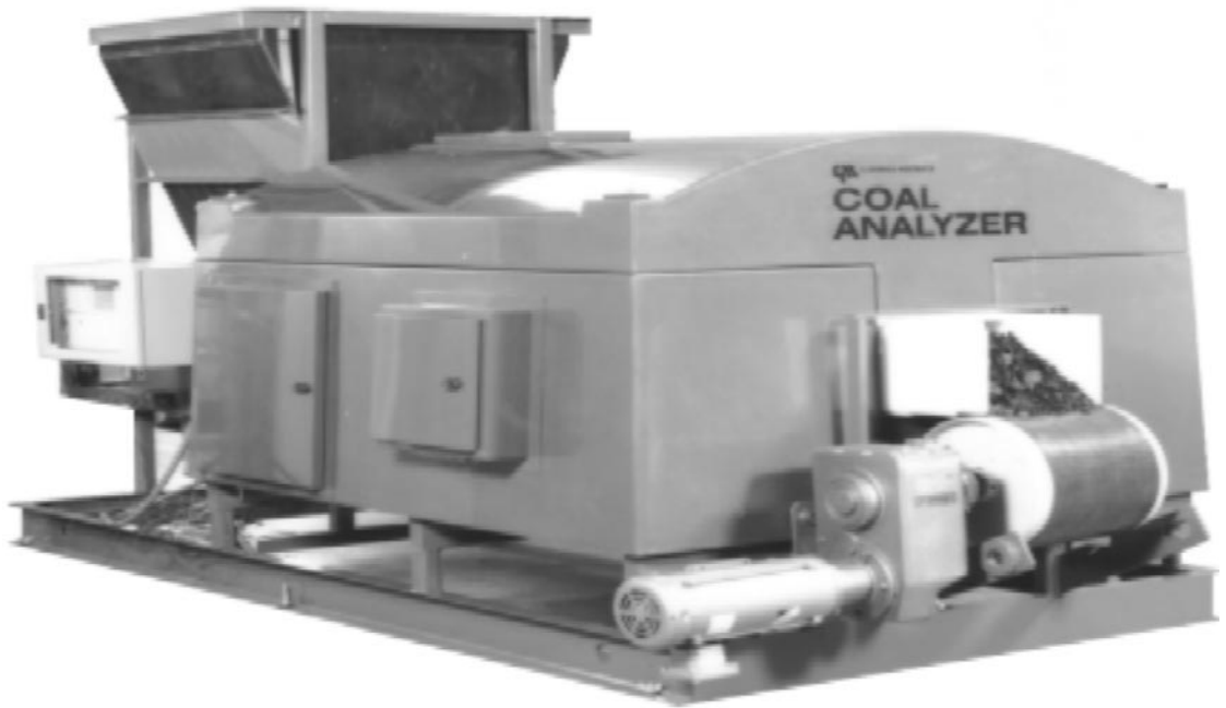
FIGURE 44 Sampled coal PGNAA analyzer can analyze 2–25 tons/h on a dedicated belt.
