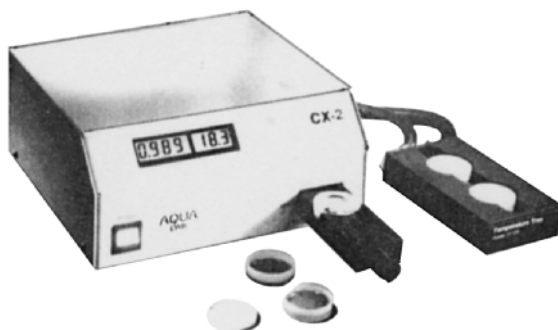
FIGURE 28 Chilled-mirror hygrometer for water activity measurements (courtesy Decagon Devices, Inc.). A chilled-mirror hygrometer specifically designed for measurement of water activity. The instrument includes special containers for the substances to be measured. Both dew point and temperature of the vapor immediately above the substance are measured and relative humidity (water activity) is calculated by a microprocessor.
