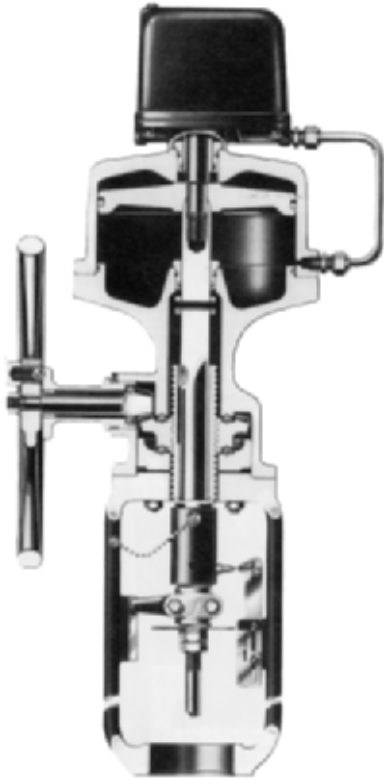
FIGURE 33 Double-acting piston actuators are a good choice if thrust requirements exceed the capability of diaphragm actuators. Piston actuators require a higher supply pressure, but they have benefits such as high stiffness and a more compact size. (Fisher Controls International, Inc.)
