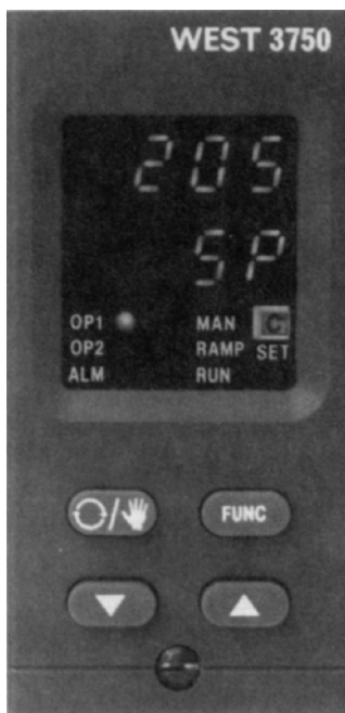
FIGURE 3 Stand-alone programmer controller in a \frac{1}{8} DIN case [96 by 48 mm (3.8 by 1.9 in.)] features a dual light-emitting diode (LED) display, and seven dedicated LEDs are used to show prompt legends during setup and the instrument status when a program is running. Full three-term control output can be offered on output 1 (heat) and output 2 (cool) with the addition of one alarm output. RS 485 serial communications option allows master-slave capabilities to profile up to 32 other similar controllers. Other features include soak hysteresis facility and dual-time-base capability to allow hour-minute or minute-second program rates. Program parameters can be revised without interruption of program. Auto-manual control allows the control of the process to be switched from automatic or closed-loop control to manual or open-loop control. Pretune and self-tune may be selected or deselected. Common applications include pottery kilns, heattreating processes, food preparation, sterilization, and environmental chambers. ( West Instruments. )
