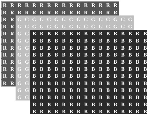
Figure 15.3 A 16 \times 12 RGB color space; each pixel has three numbers for R, G, and B
