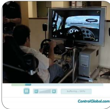
Figure 1. This realistic racing simulator uses laser-scanned images of tracks.
