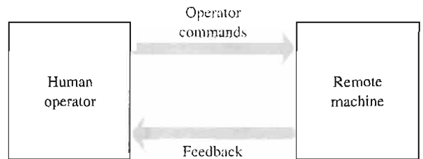
FIGURE AP6.1 Model of a teleoperated machine.
