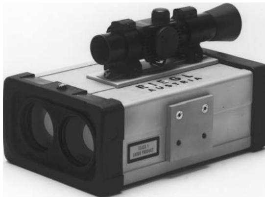
FIGURE 20.67 The Class 1 (eye-safe) LD90-3 series TOF laser rangefinder is a self-contained unit available in several versions with maximum ranges of 150–500 m under average atmospheric conditions. (Courtesy RIEGL USA.)
