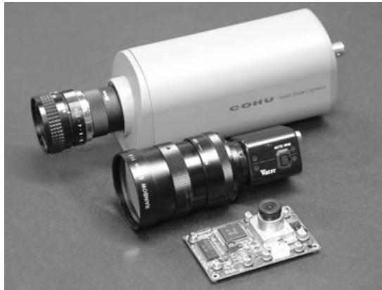
FIGURE 20.111 Three solid state cameras are shown. The nearest is an inexpensive single board camera with a CMOS sensor and 4-mm lens. The middle one is a miniature CCIR interline frame-transfer CCD camera, dwarfed by the 9.5- to 75-mm C-mount zoom lens. The rear camera is a high quality Cohu 4712 monochrome frame-transfer CCD camera fitted with a 16-mm C-mount lens and 20-mm extension tube.
