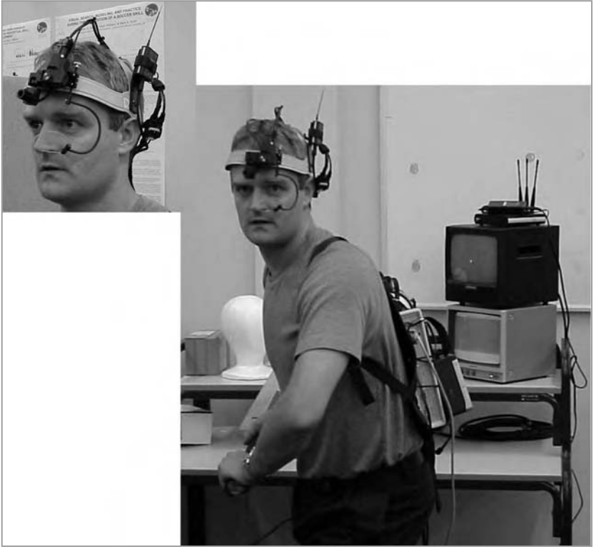
Figure 7.3 A typical head-mounted, corneal reflection system. It records the position of the pupil and corneal reflection in order to determine visual point-of-gaze during performance in simulated laboratory tasks or the 'real-world' setting
