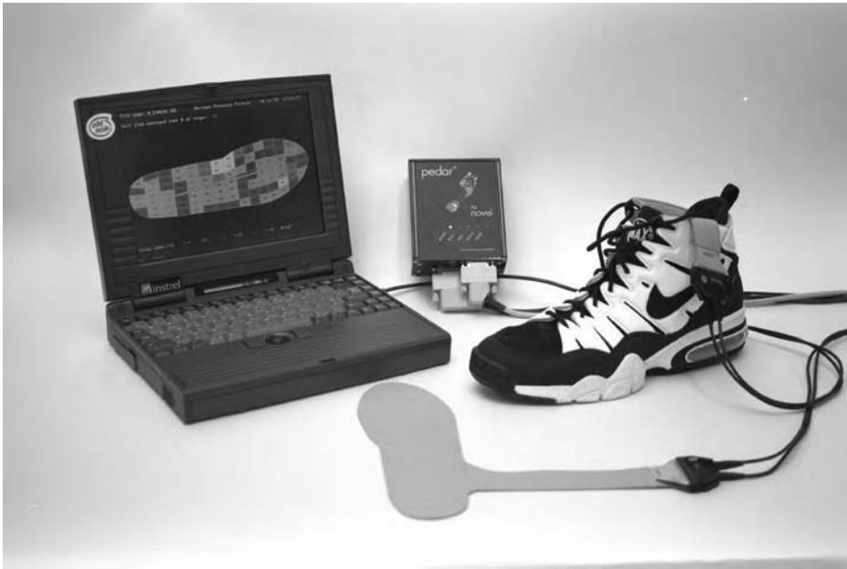
Figure 5.27 A plantar pressure insole system – Pedar™ (Novel GmbH, Munich, Germany; www.novel.de ).
