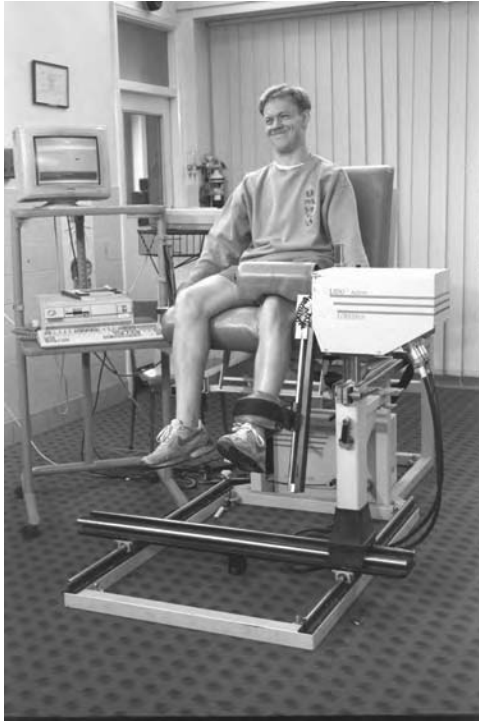
Figure 6.26 Use of an isokinetic dynamometer for: (a) knee extension; (b) elbow flexion.
