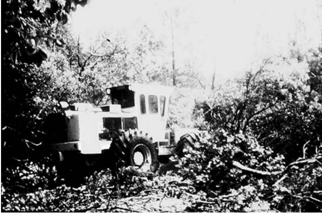
Figure 7.15 Rotary mower used for vegetation control in forestry. (Photograph by S. R. Radosevich, Oregon State University.)
