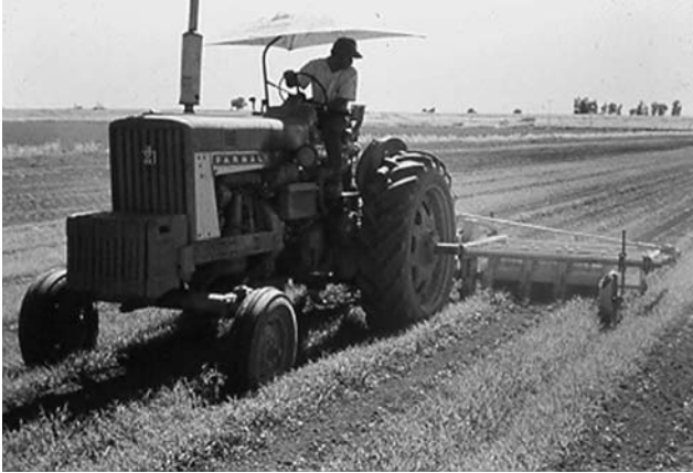
Figure 7.5 Rolling cultivator being used to control weeds in sugarbeet crop. (Photograph courtesy of R. F. Norris, University of California, Davis.)
