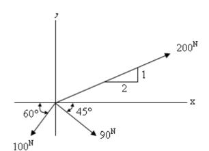
Ex (9): The screw eye in Fig. is subjected to two forces, and Determine the magnitude and direction of the resultant force.
