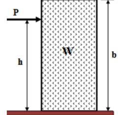
When  $h_{\rm max}>b$  then the force doesn't effect on the body , therefore , the body is not turnover .
