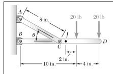
Determine the internal forces (axial force, shearing force, and bending moment) at point J of the structure indicated: Frame and loading of Prob. 6.77.
