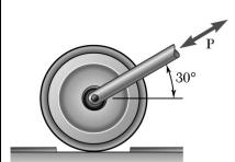
A 20-kg roller, of diameter 200 mm, which is to be used on a tile floor, is resting directly on the subflooring as shown. Knowing that the thickness of each tile is 8 mm, determine the force **P** required to move the roller onto the tiles if the roller is pulled to the right.
