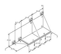
The rigid L-shaped member ABF is supported by a ball-and-socket joint at A and by three cables. For the loading shown, determine the tension in each cable and the reaction at A.
