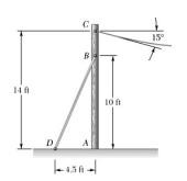
A 350-lb utility pole is used to support at C the end of an electric wire. The tension in the wire is 120 lb, and the wire forms an angle of  $15^{\circ}$  with the horizontal at C. Determine the largest and smallest allowable tensions in the guy cable BD if the magnitude of the couple at A may not exceed 200 lb · ft.
