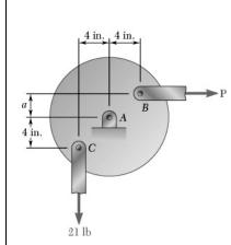
Horizontal and vertical links are hinged to a wheel, and forces are applied to the links as shown. Determine the range of values of the distance *a* for which the magnitude of the reaction at *A* does not exceed 42 lb.
