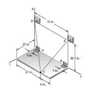
A 285-lb uniform rectangular plate is supported in the position shown by hinges A and B and by cable DCE, which passes over a frictionless hook at C. Assuming that the tension is the same in both parts of the cable, determine (a) the tension in the cable, (b) the reactions at A and B. Assume that the hinge at B does not exert any axial thrust.
