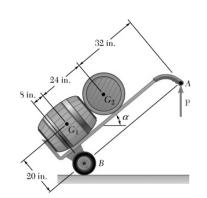
A hand truck is used to move two barrels, each weighing 80 lb. Neglecting the weight of the hand truck, determine (a) the vertical force  $\mathbf{P}$  which should be applied to the handle to maintain equilibrium when  $\alpha = 35^{\circ}$ , (b) the corresponding reaction at each of the two wheels.
