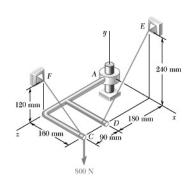
The assembly shown is welded to collar A which fits on the vertical pin shown. The pin can exert couples about the x and z axes but does not prevent motion about or along the y axis. For the loading shown, determine the tension in each cable and the reaction at A.
