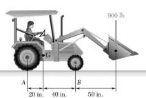
A 2100-lb tractor is used to lift 900 lb of gravel. Determine the reaction at each of the two (a) rear wheels A, (b) front wheels B.
