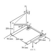
The bent rod ABEF is supported by bearings at C and D and by wire AH. Knowing that portion AB of the rod is 250 mm long, determine (a) the tension in wire AH, (b) the reactions at C and D. Assume that the bearing at D does not exert any axial thrust.
