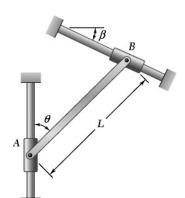
A 10-kg slender rod of length L is attached to collars which can slide freely along the guides shown. Knowing that the rod is in equilibrium and that  $\beta = 25^{\circ}$ , determine (a) the angle  $\theta$  that the rod forms with the vertical, (b) the reactions at A and B.
