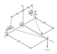
An 8-ft-long boom is held by a ball-and-socket joint at C and by two cables AD and BE. Determine the tension in each cable and the reaction at C.
