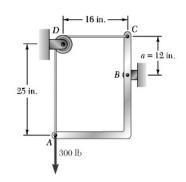
Member ABC is supported by a pin and bracket at B and by an inextensible cord at A and C and passing over a frictionless pulley at D. The tension may be assumed to be the same in portion AD and CD of the cord. For the loading shown and neglecting the size of the pulley, determine the tension in the cord and the reaction at B.
