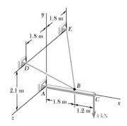
A 3-m boom is acted upon by the 4-kN force shown. Determine the tension in each cable and the reaction at the ball-and-socket joint at A.
