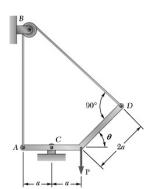
Neglecting friction, determine the tension in cable ABD and the reaction at C when  $\theta = 60^{\circ}$ .
