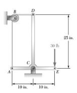
Neglecting friction, determine the tension in cable ABD and the reaction at support C.
