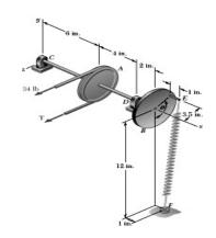
For the portion of a machine shown, the 4-in.-diameter pulley A and wheel B are fixed to a shaft supported by bearings at C and D. The spring of constant 2 lb/in. is unstretched when  $\theta = 0$ , and the bearing at C does not exert any axial force. Knowing that  $\theta = 180^{\circ}$  and that the machine is at rest and in equilibrium, determine (a) the tension T, (b) the reactions at C and D. Neglect the weights of the shaft, pulley, and wheel.
