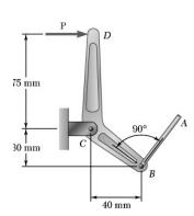
The lever BCD is hinged at C and is attached to a control rod at B. Determine the maximum force  $\mathbf{P}$  which can be safely applied at D if the maximum allowable value of the reaction at C is 500 N.
