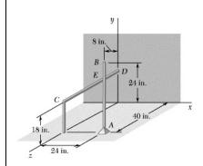
The uniform 10-lb rod AB is supported by a ball-and-socket joint at A and leans against both the rod CD and the vertical wall. Neglecting the effects of friction, determine (a) the force which rod CD exerts on AB, (b) the reactions at A and B. (Hint: The force exerted by CD on AB must be perpendicular to both rods.)
