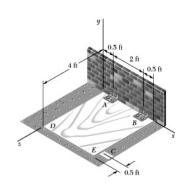
An opening in a floor is covered by a  $3 \times 4$ -ft sheet of plywood weighing 12 lb. The sheet is hinged at A and B and is maintained in a position slightly above the floor by a small block C. Determine the vertical component of the reaction (a) at A, (b) at B, (c) at C.
