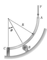
Knowing that  $\theta = 50^{\circ}$ , determine the reaction (a) at B, (b) at C.
