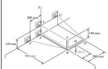
Frame ABCD is supported by a ball-and-socket joint at A and by three cables. For a=150 mm, determine the tension in each cable and the reaction at A.
