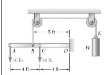
For the beam and loading shown, determine the range of values of W for which the magnitude of the couple at D does not exceed 40 lb·ft.
