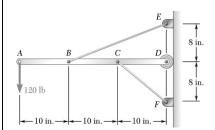
Determine the tension in each cable and the reaction at D.
