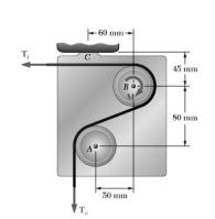
A belt passes over two 50-mm-diameter pulleys which are mounted on a bracket as shown. Knowing that M=0 and  $T_i=T_O=24$  N, determine the reaction at C.
