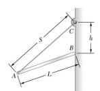
A slender rod of length L=200 mm is held in equilibrium as shown, with one end against a frictionless wall and the other end attached to a cord of length S=300 mm. Knowing that the mass of the rod is 1.5 kg, determine (a) the distance h, (b) the tension in the cord, (c) the reaction at B.
