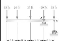
For the beam and loading shown, determine (a) the reaction at A, (b) the tension in cable BC.
