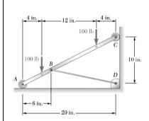
Bar AC supports two 100-lb loads as shown. Rollers A and C rest against frictionless surfaces and a cable BD is attached at B. Determine (a) the tension in cable BD, (b) the reaction at A, (c) the reaction at C.
