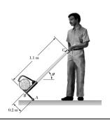
A modified peavey is used to lift a 0.2-m-diameter log of mass 36 kg. Knowing that  $\theta = 60^{\circ}$  and that the force exerted at C by the worker is perpendicular to the handle of the peavey, determine (a) the force exerted at C, (b) the reaction at A.
