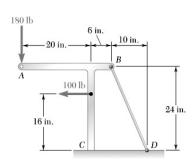
Determine the range of allowable values of the tension in wire BD if the magnitude of the couple at the fixed support C is not to exceed 75 lb·ft.
