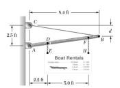
A sign is hung by two chains from mast AB. The mast is hinged at A and is supported by cable BC. Knowing that the tensions in chains DE and FH are 50 lb and 30 lb, respectively, and that d = 1.3 ft, determine (a) the tension in cable BC, (b) the reaction at A.
