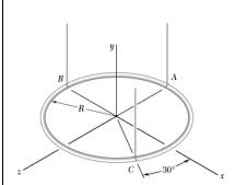
A uniform aluminum rod of weight W is bent into a circular ring of radius R and is supported by three wires as shown. Determine the tension in each wire.
