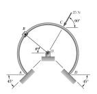
Rod ABCD is bent in the shape of a circular arc of radius 80 mm and rests against frictionless surfaces at A and D. Knowing that the collar at B can move freely on the rod, determine (a) the value of  $\theta$  for which the tension in cord OB is as small as possible, (b) the corresponding value of the tension, (c) the reactions at A and D.
