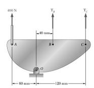
A control rod is attached to a crank at A and cords are attached at B and C. For the given force in the rod, determine the range of values of the tension in the cord at C knowing that the cords must remain taut and that the maximum allowed tension in a cord is 180 N.
