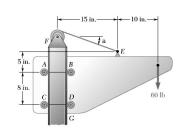
A movable bracket is held at rest by a cable attached at E and by frictionless rollers. Knowing that the width of post FG is slightly less than the distance between the rollers, determine the force exerted on the post by each roller when  $\alpha = 20^{\circ}$ .
