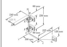
The lever AB is welded to the bent rod BCD which is supported by bearings at E and F and by cable DG. Knowing that the bearing at E does not exert any axial thrust, determine (a) the tension in cable DG, (b) the reactions at E and F.
