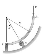
Knowing that  $\theta = 35^{\circ}$ , determine the reaction (a) at B, (b) at C.
