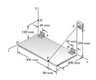
The rectangular plate shown has a mass of 15 kg and is held in the position shown by hinges A and B and cable EF. Assuming that the hinge at B does not exert any axial thrust, determine (a) the tension in the cable, (b) the reactions at A and B.
