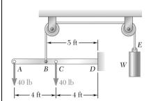
Beam AD carries the two 40-lb loads shown. The beam is held by a fixed support at D and by the cable BE which is attached to the counter-weight W. Determine the reaction at D when (a) W = 100 lb, (b) W = 90 lb.
