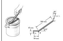
To remove the lid from a 5-gallon pail, the tool shown is used to apply an upward and radially outward force to the bottom inside rim of the lid. Assuming that the rim rests against the tool at *A* and that a 100-N force is applied as indicated to the handle, determine the force acting on the rim.
