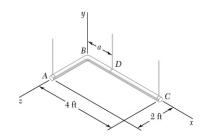
Two steel pipes AB and BC, each having a weight per unit length of 5 lb/ft, are welded together at B and are supported by three wires. Knowing that a = 1.25 ft, determine the tension in each wire.
