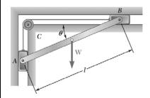
A slender rod AB, of weight W, is attached to blocks A and B, which move freely in the guides shown. The blocks are connected by an elastic cord which passes over a pulley at C. (a) Express the tension in the cord in terms of W and  $\theta$ . (b) Determine the value of  $\theta$  for which the tension in the cord is equal to 3W.
