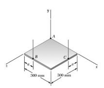
The 10-kg square plate shown is supported by three vertical wires. Determine (a) the tension in each wire when a = 100 mm, (b) the value of a for which tensions in the three wires are equal.
