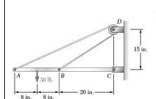
Neglecting friction and the radius of the pulley, determine (a) the tension in cable ABD, (b) the reaction at C.
