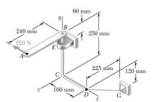
The lever AB is welded to the bent rod BCD which is supported by bearing E and by cable DG. Assuming that the bearing can exert an axial thrust and couples about axes parallel to the x and z axes, determine (a) the tension in cable DG, (b) the reaction at E.
