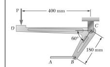
The required tension in cable AB is 800 N. Determine (a) the vertical force **P** which must be applied to the pedal, (b) the corresponding reaction at C.
