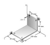
Two rectangular plates are welded together to form the assembly shown. The assembly is supported by ball-and-socket joints at B and D and by a ball on a horizontal surface at C. For the loading shown, determine the reaction at C.
