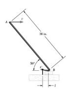
To remove a nail, a small block of wood is placed under a crowbar, and a horizontal force **P** is applied as shown. Knowing that l = 3.5 in. and P = 30 lb, determine the vertical force exerted on the nail and the reaction at B.
