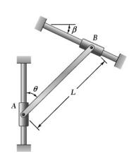
A slender rod of length L and weight W is attached to collars which can slide freely along the guides shown. Knowing that the rod is in equilibrium, derive an expression for the angle  $\theta$  in terms of the angle  $\beta$ .
