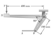
Determine the maximum tension which can be developed in cable AB if the maximum allowable value of the reaction at C is 1000 N.
