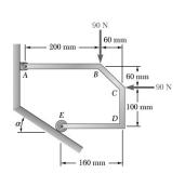
For the frame and loading shown, determine the reactions at A and E when (a)  $\alpha = 30^{\circ}$ , (b)  $\alpha = 45^{\circ}$ .
