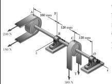
Two transmission belts pass over sheaves welded to an axle supported by bearings at B and D. The sheave at A has a radius of 50 mm, and the sheave at C has a radius of 40 mm. Knowing that the system rotates with a constant rate, determine (a) the tension T, (b) the reactions at B and D. Assume that the bearing at D does not exert any axial thrust and neglect the weights of the sheaves and the axle.
