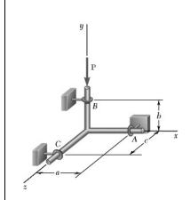
Three rods are welded together to form a "corner" which is supported by three eyebolts. Neglecting friction, determine the reactions at A, B, and C when P = 240 N, a = 120 mm, b = 80 mm, and c = 100 mm.
