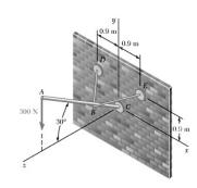
The 3-m flagpole AC forms an angle of  $30^{\circ}$  with the z axis. It is held by a ball-and-socket joint at C and by two thin braces BD and BE. Knowing that the distance BC is 0.9 m, determine the tension in each brace and the reaction at C.
