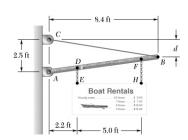
A sign is hung by two chains from mast AB. The mast is hinged at A and is supported by cable BC. Knowing that the tensions in chains DE and FH are 30 lb and 20 lb, respectively, and that d = 1.54 ft, determine (a) the tension in cable BC, (b) the reaction at A.
