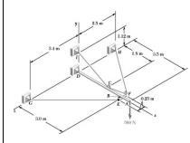
Two steel pipes ABCD and EBF are welded together at B to form the boom shown. The boom is held by a ball-and-socket joint at D and by two cables EG and ICFH; cable ICFH passes around frictionless pulleys at C and F. For the loading shown, determine the tension in each cable and the reaction at D.
