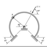
Rod ABCD is bent in the shape of a circular arc of radius 80 mm and rests against frictionless surfaces at A and D. Knowing that the collar at B can move freely on the rod and that  $\theta = 45^{\circ}$ . determine (a) the tension in cord OB, (b) the reactions at A and D.
