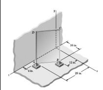
A uniform 20  $\times$  30-in. steel plate ABCD weighs 85 lb and is attached to ball-and-socket joints at A and B. Knowing that the plate leans against a frictionless vertical wall at D, determine (a) the location of D, (b) the reaction at D.
