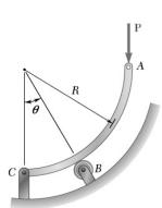
Rod ABC is bent in the shape of a circular arc of radius R. Knowing that  $\theta = 50^{\circ}$ , determine the reaction (a) at B, (b) at C.
