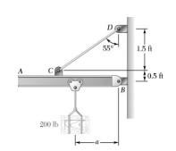
A 200-lb crate is attached to the trolley-beam system shown. Knowing that a = 1.5 ft, determine (a) the tension in cable CD, (b) the reaction at B.
