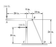
Knowing that the tension in wire *BD* is 300 lb, determine the reaction at fixed support *C* for the frame shown.
