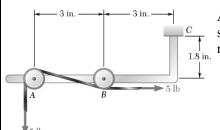
A tension of 5 lb is maintained in a tape as it passes the support system shown. Knowing that the radius of each pulley is 0.4 in., determine the reaction at C.
