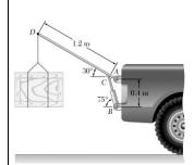
A small hoist is mounted on the back of a pickup truck and is used to lift a 120-kg crate. Determine (a) the force exerted on the hoist by the hydraulic cylinder BC, (b) the reaction at A.
