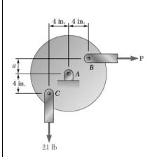
Horizontal and vertical links are hinged to a wheel, and forces are applied to the links as shown. Knowing that a = 3.0 in., determine the value of P and the reaction at A.
