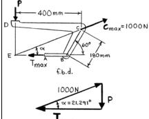
$$\alpha = \tan^{-1} \left[ \frac{(180 \text{ mm})\sin 60^{\circ}}{400 \text{ mm}} \right] = 21.291^{\circ}$$
