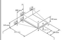
Frame ABCD is supported by a ball-and-socket joint at A and by three cables. Knowing that the 350-N load is applied at D (a = 300 mm), determine the tension in each cable and the reaction at A.
