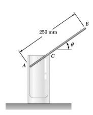
A uniform slender rod of mass 5 g and length 250 mm is balanced on a glass of inner diameter 70 mm. Neglecting friction, determine the angle  $\theta$ corresponding to equilibrium.
