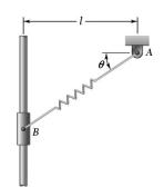
A collar B of weight W can move freely along the vertical rod shown. The constant of the spring is k, and the spring is unstretched when  $\theta = 0$ . (a) Derive an equation in  $\theta$ , W, k, and l which must be satisfied when the collar is in equilibrium. (b) Knowing that W = 3 lb, l = 6 in., and k = 8 lb/ft, determine the value of  $\theta$  corresponding to equilibrium.
