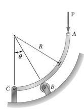
Rod ABC is bent in the shape of a circular arc of radius R. Knowing that  $\theta = 35^{\circ}$ , determine the reaction (a) at B, (b) at C.
