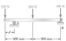
The maximum allowable value of each of the reactions is 360 N. Neglecting the weight of the beam, determine the range of values of the distance *d* for which the beam is safe.
