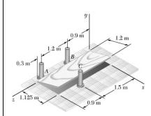
A  $1.2 \times 2.4$ -m sheet of plywood having a mass of 17 kg has been temporarily placed among three pipe supports. The lower edge of the sheet rests on small collars A and B and its upper edge leans against pipe C. Neglecting friction at all surfaces, determine the reactions at A, B, and C.
