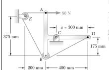
Member ABCD is supported by a pin and bracket at C and by an inextensible cord attached at A and D and passing over frictionless pulleys at B and E. Neglecting the size of the pulleys, determine the tension in the cord and the reaction at C.
