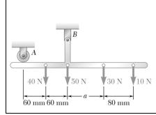
For the bracket and loading of Problem 4.5, determine the smallest distance a if the bracket is not to move.
