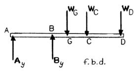
$$W_G = m_G g = (65 \text{ kg})(9.81 \text{ m/s}^2) = 637.65 \text{ N}$$
