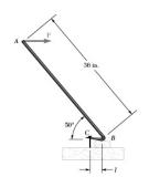
To remove a nail, a small block of wood is placed under a crowbar, and a horizontal force **P** is applied as shown. Knowing that the maximum vertical force needed to extract the nail is 600 lb and that the horizontal force **P** is not to exceed 65 lb, determine the largest acceptable value of distance *l*.
