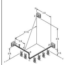
To water seedlings, a gardener joins three lengths of pipe, AB, BC, and CD, fitted with spray nozzles and suspends the assembly using hinged supports at A and D and cable EF. Knowing that the pipe weighs 0.85 lb/ft, determine the tension in the cable.
