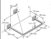
The bent rod ABDE is supported by ball-and-socket joints at A and E and by the cable DF. If a 600-N load is applied at C as shown, determine the tension in the cable.
