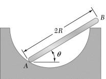
A uniform rod AB of weight W and length 2R rests inside a hemispherical bowl of radius R as shown. Neglecting friction determine the angle  $\theta$  corresponding to equilibrium.
