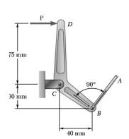
The lever BCD is hinged at C and is attached to a control rod at B. If P = 200 N, determine (a) the tension in rod AB, (b) the reaction at C.
