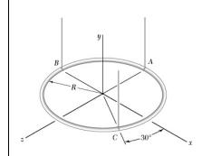
A uniform aluminum rod of weight W is bent into a circular ring of radius R and is supported by three wires as shown. A small collar of weight W' is then placed on the ring and positioned so that the tensions in the three wires are equal. Determine (a) the position of the collar, (b) the value of W', (c) the tension in the wires.
