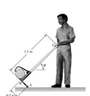
A modified peavey is used to lift a 0.2-m-diameter log of mass 36 kg. Knowing that  $\theta = 45^{\circ}$  and that the force exerted at C by the worker is perpendicular to the handle of the peavey, determine (a) the force exerted at C, (b) the reaction at A.
