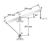
A lever AB is hinged at C and is attached to a control cable at A. If the lever is subjected to a 300-N vertical force at B, determine (a) the tension in the cable, (b) the reaction at C.
