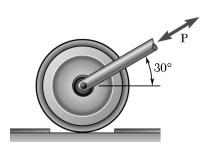
A 20-kg roller, of diameter 200 mm, which is to be used on a tile floor, is resting directly on the subflooring as shown. Knowing that the thickness of each tile is 8 mm, determine the force **P** required to move the roller onto the tiles if the roller is pushed to the left.
