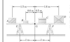
Four boxes are placed on a uniform 14-kg wooden plank which rests on two sawhorses. Knowing that the masses of boxes B and D are 4.5 kg and 45 kg, respectively, determine the range of values of the mass of box A so that the plank remains in equilibrium when box C is removed.
