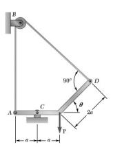
Neglecting friction, determine the tension in cable *ABD* and the reaction at *C* when  $\theta = 30^{\circ}$ .
