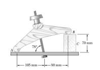
The clamp shown is used to hold the rough workpiece C. Knowing that the maximum allowable compressive force on the workpiece is 200 N and neglecting the effect of friction at A, determine the corresponding (a) reaction at B, (b) reaction at A, (c) tension in the bolt.
