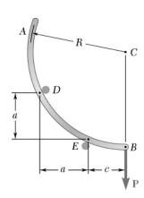
Rod AB is bent into the shape of a circular arc and is lodged between two pegs D and E. It supports a load  $\mathbf{P}$  at end B. Neglecting friction and the weight of the rod, determine the distance c corresponding to equilibrium when a=1 in. and R=5 in.
