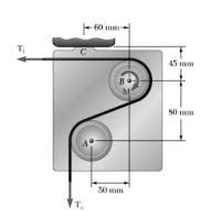
A belt passes over two 50-mm-diameter pulleys which are mounted on a bracket as shown. Knowing that  $M = 0.40 \text{ N} \cdot \text{m}$  m and that  $T_i$  and  $T_O$  are equal to 32 N and 16 N, respectively, determine the reaction at C.
