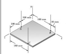
The  $200 \times 200$ -mm square plate shown has a mass of 25 kg and is supported by three vertical wires. Determine the mass and location of the lightest block which should be placed on the plate if the tensions in the three cables are to be equal.
