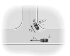
$$\mathbf{v_{BA}} = \mathbf{v_{Bv}} - \mathbf{v_{Av}} \qquad \mathbf{v_{BA}} = \begin{pmatrix} 20\\17.321 \end{pmatrix} \frac{\mathrm{mi}}{\mathrm{hr}} \qquad |\mathbf{v_{BA}}| = 26.458 \frac{\mathrm{mi}}{\mathrm{hr}}$$
