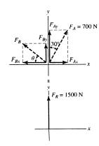
**2-44.** Determine the magnitude and orientation, measured counterclockwise from the positive y axis, of the resultant force acting on the bracket, if  $F_B = 600$  N and  $\theta = 20^\circ$ .
