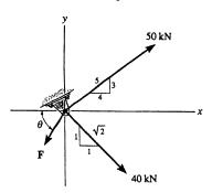
$$\stackrel{+}{\to} F_{Rx} = \Sigma F_x; \qquad F_{Rx} = 50(\frac{4}{5}) + \frac{1}{\sqrt{2}}(40) - 20 \cos 60^\circ = 58.28 \text{ kN}$$
