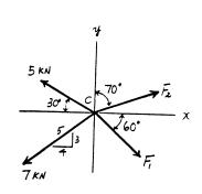
**3-6.** The members of a truss are pin-connected at joint O. Determine the magnitude of  $\mathbf{F}_1$  and its angle  $\theta$  for equilibrium. Set  $F_2 = 6$  kN.
