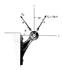
Scalar Notation: Suming the force components algebraically, we have
