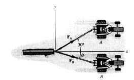
${\it Parallelogram\ Law:}$  The parallelogram law of addition is shown in Fig. (a).
