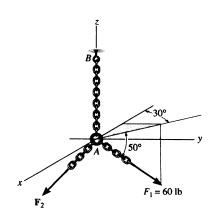
**2-73.** The bracket is subjected to the two forces shown. Express each force in Cartesian vector form and then determine the resultant force  $\mathbf{F}_R$ . Find the magnitude and coordinate direction angles of the resultant force.
