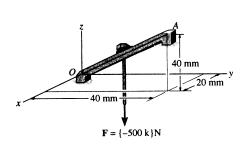
**\*2-120.** Determine the projection of the force  ${\bf F}$  along the pole.
