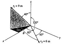
$$r_1 = 9(\sin 40^{\circ} \cos 30^{\circ} i - \sin 40^{\circ} \sin 30^{\circ} j + \cos 40^{\circ} k)$$
