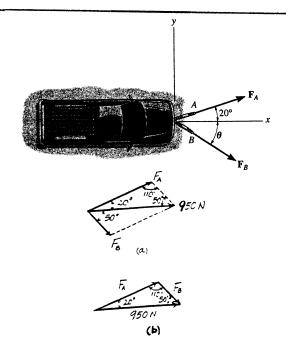
**2-21.** The truck is to be towed using two ropes. If the resultant force is to be 950 N, directed along the positive x axis, determine the magnitudes of forces  $\mathbf{F}_A$  and  $\mathbf{F}_B$  acting on each rope and the angle of  $\theta$  of  $\mathbf{F}_B$  so that the magnitude of  $\mathbf{F}_B$  is a *minimum*.  $\mathbf{F}_A$  acts at 20° from the x axis as shown.
