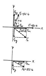
\*2-57. If  $F_2 = 150$  lb and  $\theta = 55^\circ$ , determine the magnitude and orientation, measured clockwise from the positive x axis, of the resultant force of the three forces acting on the bracket.
