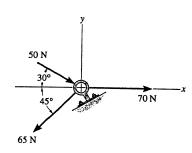
$$\stackrel{+}{\to} F_{R_x} = \Sigma F_x; \qquad F_{R_x} = 70 + 50\cos 30^\circ - 65\cos 45^\circ = 67.34 \text{ N}$$
