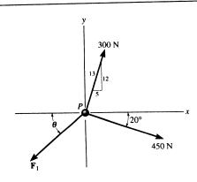
\*3-4. Determine the magnitude and angle  $\theta$  of **F** so that the particle is in equilibrium.
