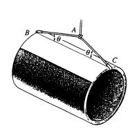
**3-10.** The 500-lb crate is hoisted using the ropes AB and AC. Each rope can withstand a maximum tension of 2500 lb before it breaks. If AB always remains horizontal, determine the smallest angle  $\theta$  to which the crate can be hoisted.
