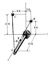
2-128. If F has a magnitude of 55 lb, determine the magnitude of its projected component acting along the x axis and along cable AC.
