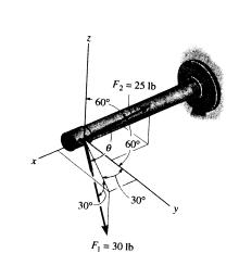
**2-126.** Determine the angle  $\theta$  between the two cables attached to the pipe.
