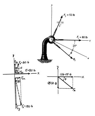
2-58. Determine the magnitude of force F so that the resultant force of the three forces is as small as possible. What is the magnitude of the resultant force?
