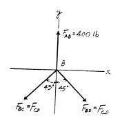
3-13. Determine the stretch in each spring for equilibrium of the 2-kg block. The springs are shown in the equilibrium position.
