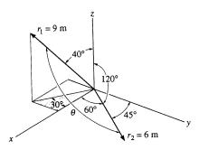
$$r_1 = 9 (\sin 40^{\circ} \cos 30^{\circ} i - \sin 40^{\circ} \sin 30^{\circ} j + \cos 40^{\circ} k)$$
