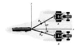
**Parallelogram Law:** In order to produce a minimum force  $\mathbf{F}_B$ ,  $\mathbf{F}_B$  has to act perpendicular to  $\mathbf{F}_A$ . The parallelogram law of addition is shown in Fig. (a).
