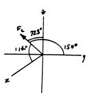
\*2-60. The cable at the end of the crane boom exerts a force of 250 lb on the boom as shown. Express F as a Cartesian vector.
