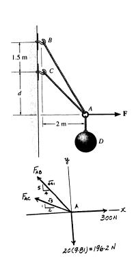
**3-21.** The ball D has a mass of 20 kg. If a force of F = 100 N is applied horizontally to the ring at A, determine the largest dimension d so that the force in cable AC is zero.
