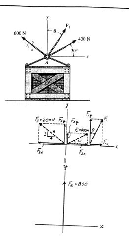
**2-38.** Determine the magnitude and direction measured counterclockwise from the positive x axis of the resultant force of the three forces acting on the ring A. Take  $F_1 = 500 \text{ N}$  and  $\theta = 20^\circ$ .
