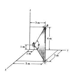
\*2-116. Determine the length of side BC of the triangular plate. Solve the problem by finding the magnitude of  $\mathbf{r}_{BC}$ ; then check the result by first finding  $\theta$ ,  $r_{AB}$ , and  $r_{AC}$  and then use the cosine law.
