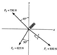
$$\stackrel{+}{\to} F_{R_x} = \Sigma F_x; \qquad F_{R_x} = \frac{4}{5}(850) - 625 \sin 30^\circ - 750 \sin 45^\circ = -162.8 \text{ N}$$
