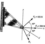
$$\stackrel{+}{\to} F_{Rx} = \Sigma F_x; \quad 1000 \cos 30^\circ = 200 + 450 \cos 45^\circ + F_1 \cos(\theta + 30^\circ)$$
