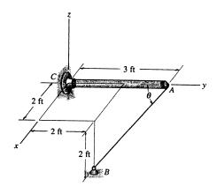
**2-114.** The force  $\mathbf{F} = \{25\mathbf{i} - 50\mathbf{j} + 10\mathbf{k}\}$  N acts at the end A of the pipe assembly. Determine the magnitude of the components  $\mathbf{F}_1$  and  $\mathbf{F}_2$  which act along the axis of AB and perpendicular to it.
