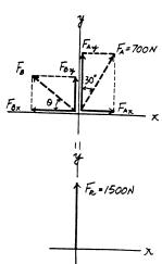
**2-42.** Solve Prob. 2-22 by summing the rectangular or x, y components of the forces to obtain the resultant force.
