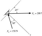
$+ F_{Rx} = \Sigma F_x;$   $F_{Rx} = -150\cos 30^{\circ} + 200\sin 45^{\circ} = 11.518 \text{ N}$
