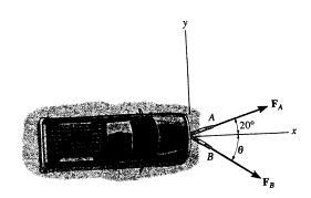
Parallelogram Law: In order to produce a minimum force  $F_B$ ,  $F_B$  has to act perpendicular to  $F_A$ . The parallelogram law of addition is shown in Fig. (a).
