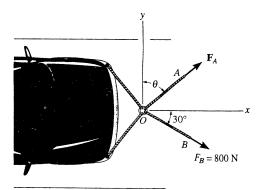
**2-50.** Determine the magnitude and direction, measured counterclockwise from the positive x axis, of the resultant force acting on the ring at O, if  $F_A = 750$  N and  $\theta = 45^{\circ}$ .
