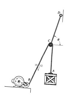
**3-19.** The cords BCA and CD can each support a maximum load of 100 lb. Determine the maximum weight of the crate that can be hoisted at constant velocity, and the angle  $\theta$  for equilibrium.
