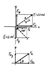
2-34. Determine the magnitude of the resultant force and its direction, measured counterclockwise from the positive x axis.
