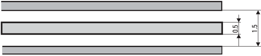
Figure 7.1 The stripline cross section. The center conductor is a 0.5-mm metal sheet of variable width and the air gap above and below it is 0.5 mm as well [3].
