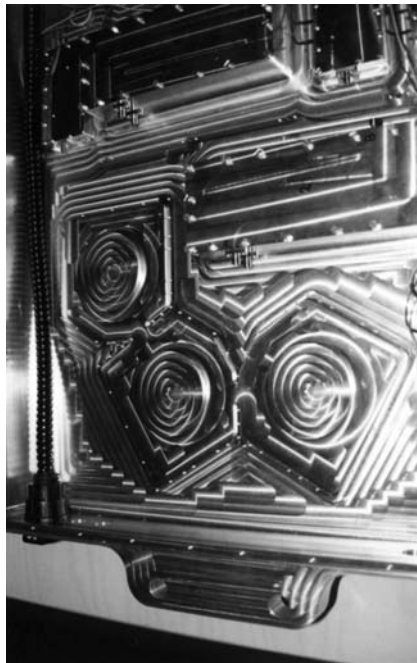
Figure 9.12 The lane on which the milling tool has moved is easy to see from the surface, but the surface roughness is even better than R_a = 1.6 \mu\text{m} .
