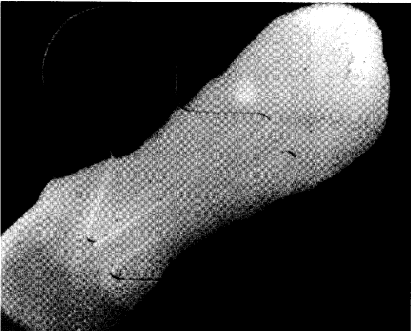
Fig. 4 The first metal-oxide-semiconductor field-effect transistor. 13 (Photograph courtesy of Bell Laboratories.)
